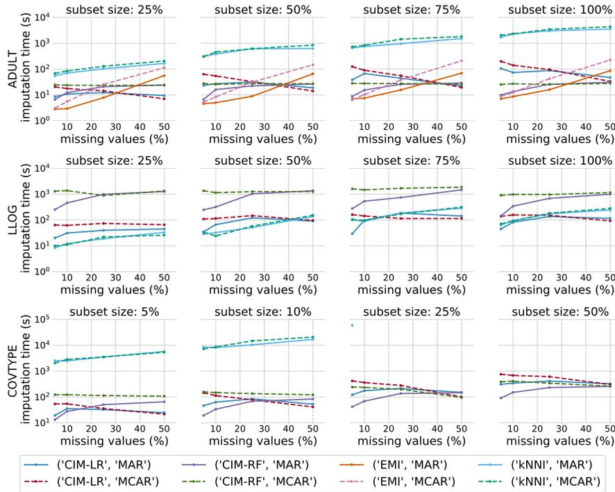
**Figure 4.4:** Scalability test results for CIM, EMI and  $\kappa$ NNI. CIM imputation time decreases with larger missing values ratios, while EMI and  $\kappa$ NNI are weak against large data set sizes and ratio of missing values.
