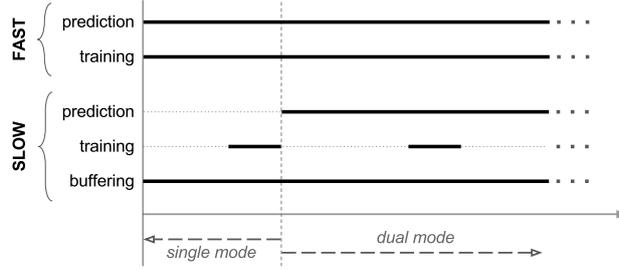
**Figure 5.2:** FSC operation. In *single-mode*, the FAST model is used for prediction while SLOW is buffering the data. In *dual-mode*, both models predict each sample but only one is selected based on their recent performance. SLOW models are replaced in presence of concept drift.
