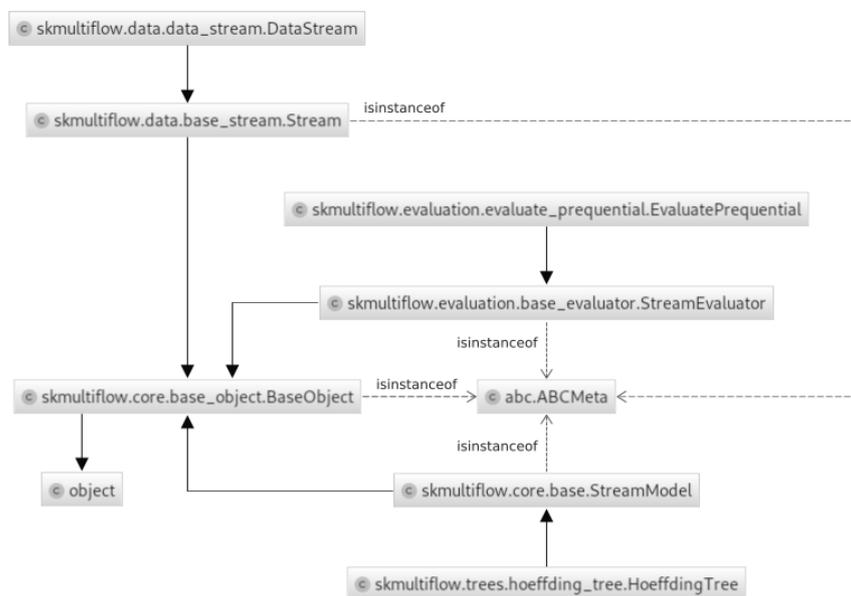
Figure 7.1: Class hierarchy within scikit-multiflow. This example shows instances of a `StreamModel` (`HoeffdingTree`), a `Stream` (`DataStream`) and a `StreamEvaluator` (`EvaluatePrequential`).
