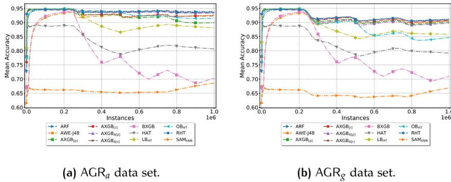
Figure 6.3: Example of the impact of concept drift on the mean performance of models compared in our tests. The AGR<sub>a</sub>, Figure 6.3a, and AGR<sub>g</sub>, Figure 6.3b, data sets contain drifts at the 25%, 50% and 75% of the stream.
