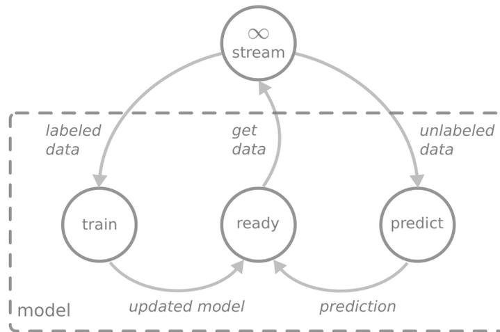
**Figure 2.1:** Stream supervised learning. A data stream is an infinite source of data whereas a predictive model transitions from *ready* to either *train* or *predict* and back. Labeled data is used to train/update the model. If data is unlabeled, then the model predicts the corresponding target value (class label in the case of classification).
