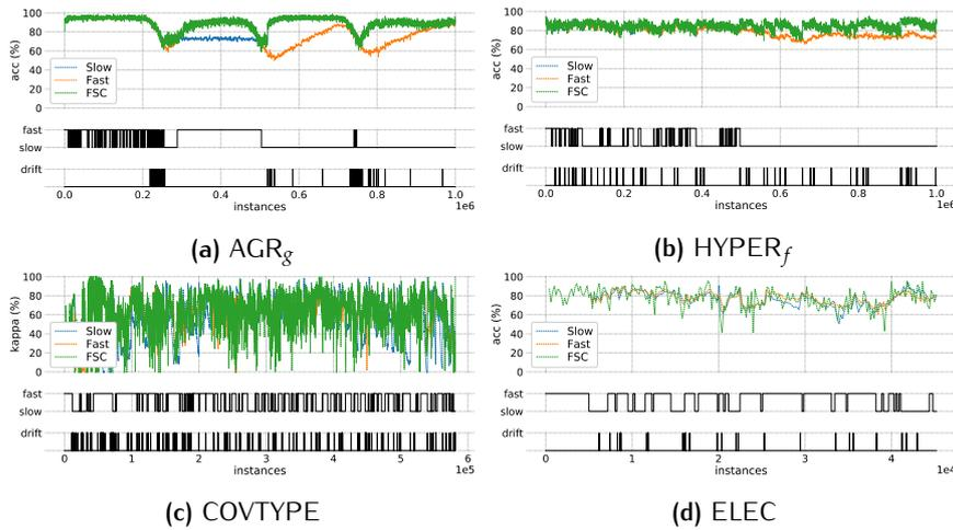
Figure 5.5: Current (sliding) performance of  $FSC_{ff}$  with fading factors (green) vs FAST (orange) vs SLOW (blue). Notice that using fading factors results in less transitions between models.
