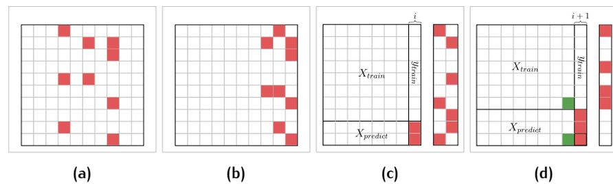
**Figure 4.1:** CIM Steps. (4.1a) Original data with missing values marked in red. (4.1b) Updated positions after sorting attributes by count of missing values. (4.1c-4.1d) Imputation iterations, repeated until data set is complete. Imputed values in green are used in following iterations of the algorithm.
