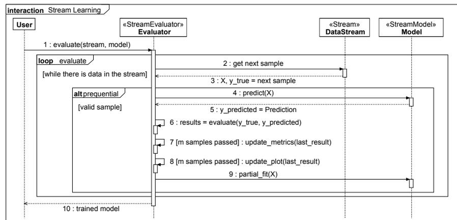
**Figure 7.2:** Training and testing a stream model using scikit-multiflow. This sequence corresponds to prequential evaluation.
