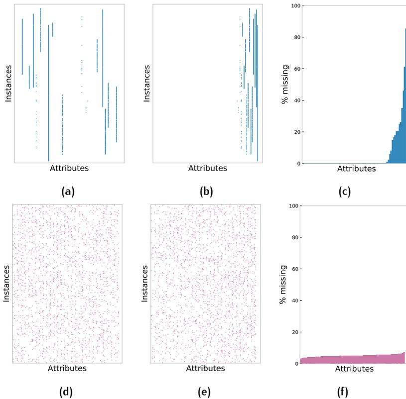
**Figure A.1:** Difference between MAR (top) and MCAR (bottom) data distributions. Plots correspond to the same data set (Music) with 5% missing values. Figures A.1a and A.1d show original position of missing values (dots). Figures A.1b and A.1e show the updated positions after initial column-wise sorting performed by CIM. Figures A.1c and A.1f are missing values histograms after sorting.
