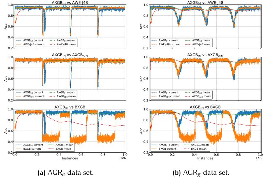
**Figure 6.4:** Performance of  $AXGB_{[r]}$  vs AWE-J48,  $AXGB_{A[r]}$  and BXGB. Values marked as *current* correspond to accuracy on a sliding window of 200 samples.
