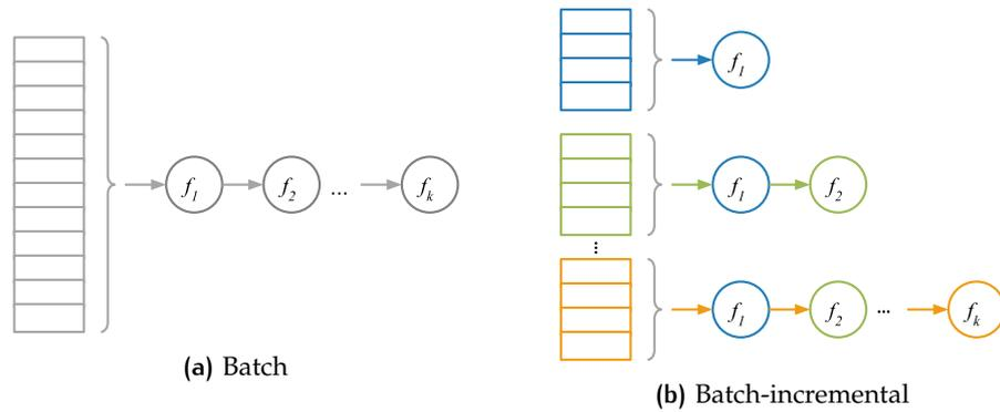
**Figure 6.1:** Ensemble creation strategies. The standard batch approach, Figure 6.1a, uses all available data to create all the members of the ensemble. On the other hand, the batch-incremental approach, Figure 6.1b, uses data windows to incrementally create the members of the ensemble as data becomes available.
