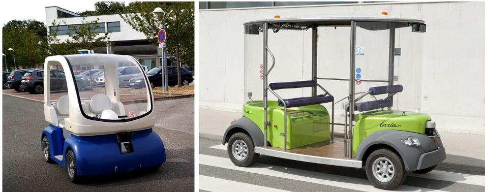
Figure 2.14 – INRIA’s Cybercars: Cycab (left) and Cybus (right)
