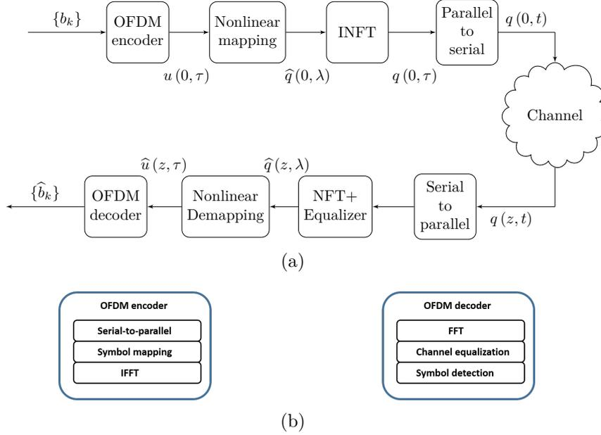
**Figure 2.10:** The architecture of NFD transmission system (a) and (b) the corresponding DSP.
