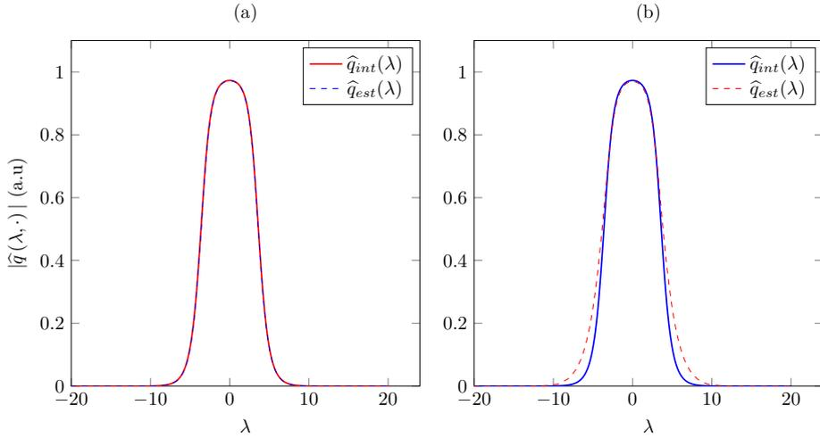
**Figure 4.9:** The NFT continuous spectrum of a lossless and lossy transmission where the later approximated by the LPA method.
