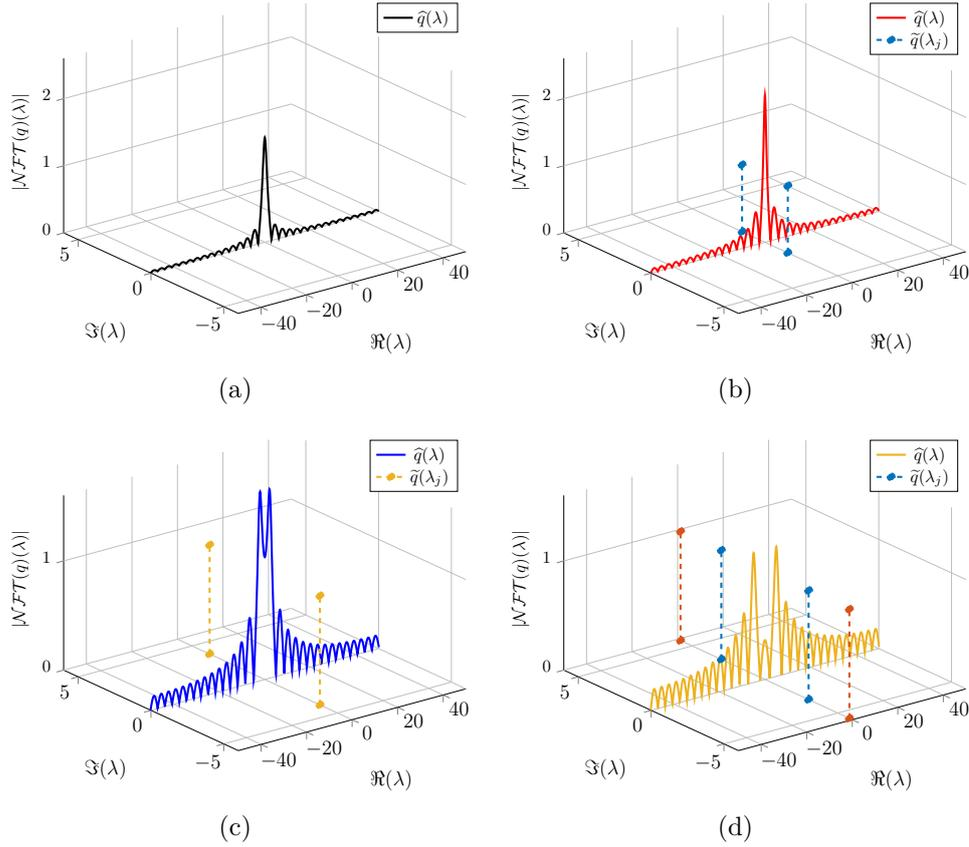
**Figure 2.4:** Illustration of the NFT of a simple un-modulated rectangular pulse. The absolute value of the continuous spectrum of a rectangular pulse  $q(t) = A * rect(t)$ , (a), evolves from a simple sinc-type for (b)  $A=1$ , to more complicated shapes for (c)  $A=4$ , and (d)  $A=6$ .
