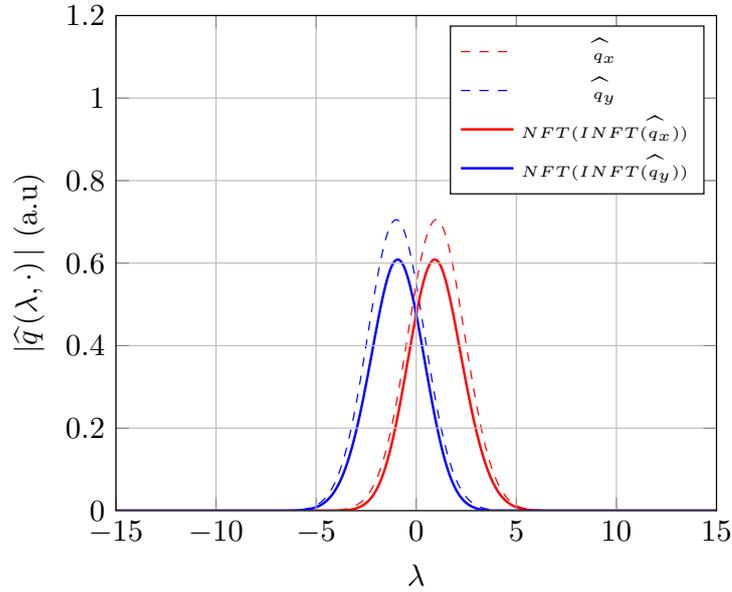
**Figure 2.11:** The numerical accuracy of a dual-polarization NFT-INFT pair for a dual polarization signal which given by a shifted Gaussian shaped initial spectrum  $\widehat{\mathbf{q}} = [\widehat{q}_x, \widehat{q}_y]$  and  $NFT(INFT(\widehat{\mathbf{q}}))$  at high power. For a fixed sample size, the accuracy of algorithm decreases at large amplitudes (after [83]).
