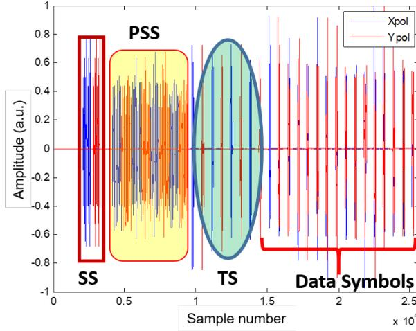
**Figure 3.15:** Data structure of real part of 16QAM PDM-NFDM/OFDM.
