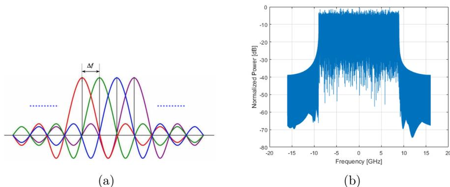
**Figure 3.2:** Principle of OFDM and its spectrum. (a) Theoretical overlapping and orthogonal subcarriers, (b) experimental Nyquist bandwidth of OFDM.
