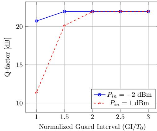
**Figure 4.14:** Simulation result of a B2B Q-factor performance as a function of NGI for NFDM transmissions with input power of  $-4$  dBm and  $-1$  dBm.
