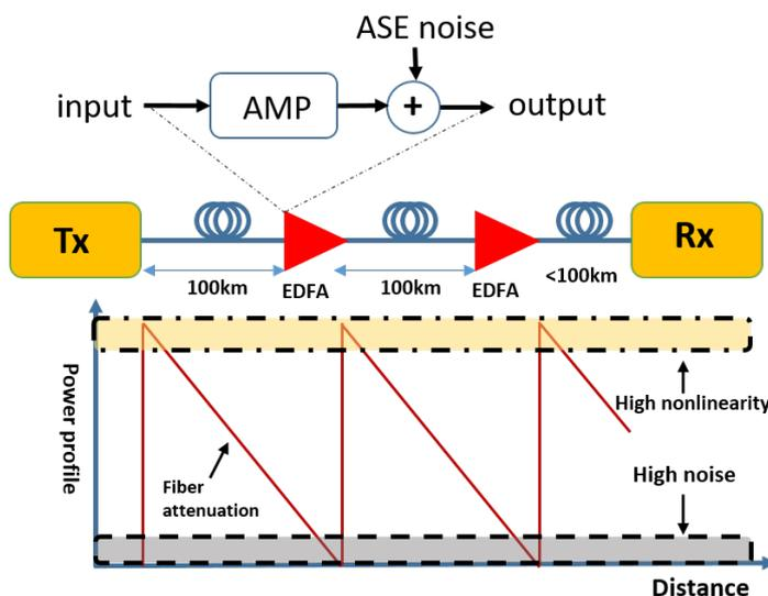
**Figure 1.7:** Schematic representation of lumped amplification using EDFAs.
