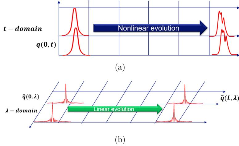
**Figure 2.9:** Illustration of nonlinear pulse evolution in a nonlinear dispersive channel in, (a) temporal domain where the input-output mapping become complex; and (b) nonlinear frequency domain where the nonlinear spectral amplitude evolve in linear and trivial manner.
