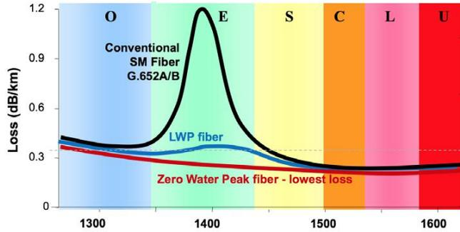
**Figure 1.5:** Attenuation curve of conventional G-652 fibers.
