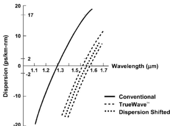
**Figure 1.6:** Dispersion curves of various single-mode fibers [37].
