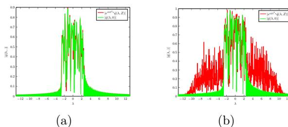
**Figure 4.5:** Illustration of the NFDM transmission performance in a noisy and noise free transmissions. The input and output continuous spectral amplitude  $\hat{q}(\cdot, \lambda)$  is shown here in the case of: (a) a noise free, and (b) a noisy optical link,
