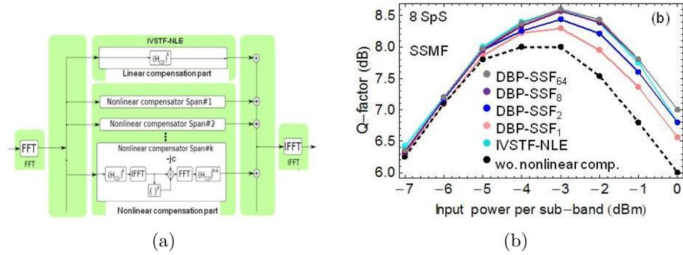
**Figure 1.12:** (a)Block diagram of IVSTF-NLEs equalizer; and (b) Q-factor vs. input power performance improvement obtained for 400 Gb/s without/with IVSTF-NLEs and DBP-SSFM<sub>1,2,8,64</sub> in SSMF (after [59]).
