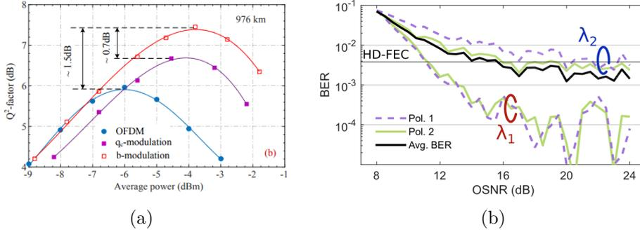
**Figure 3.1:** Illustration of NFDM optical transmissions. (a) A Q-factor as a function of the launch power when modulating the continuous spectrum [105]; (b) BER performance as a function of OSNR for discrete spectrum modulation in a dual-polarization configuration [84].
