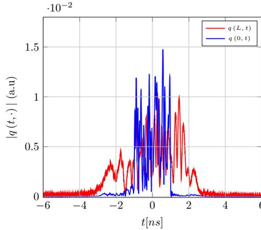
**Figure 3.6:** Signal broadening due to dispersion in NFDM transmission over 1600 km fiber link.
