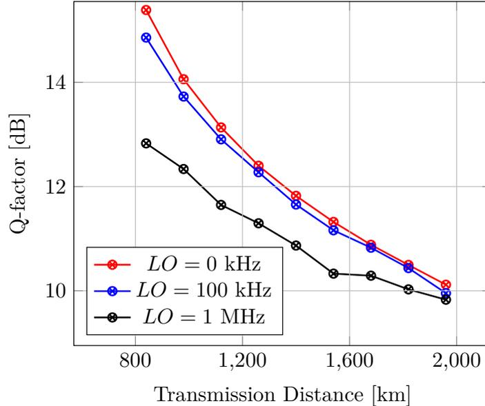
**Figure 4.13:** Q-factor performance versus transmission distance (no ASE noise is considered).
