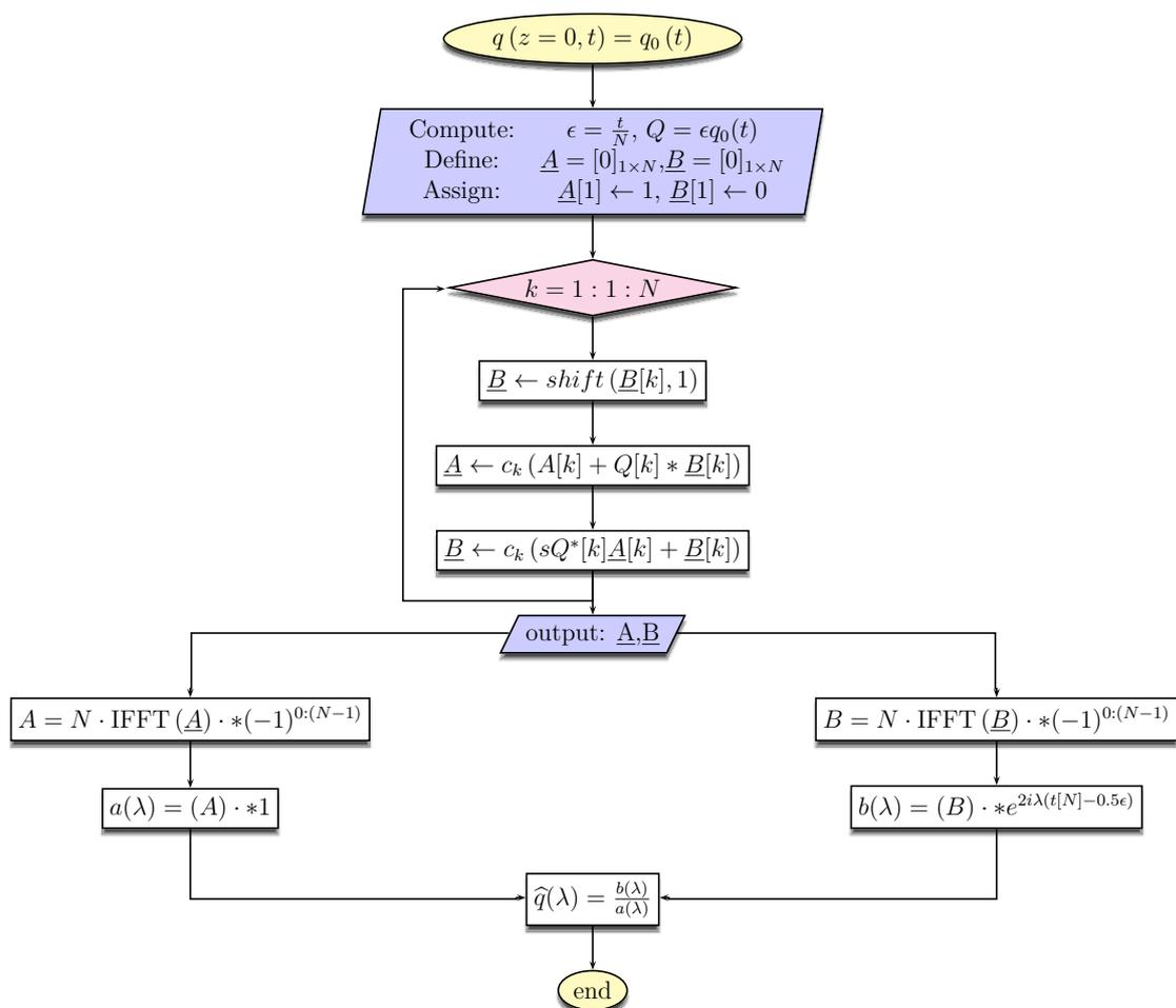
**Figure 2.7:** Flow chart of NFT algorithm implementation (after [75]).
