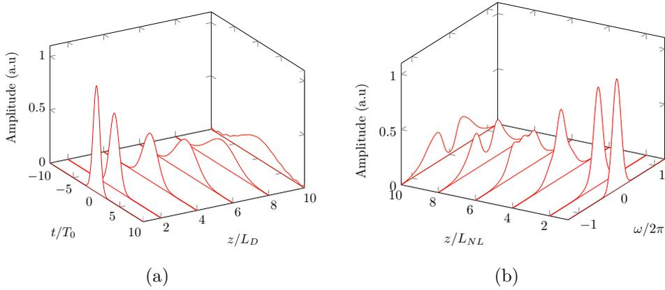
**Figure 1.8:** Illustration of pulse broadening effect due to GVD (a), and (b) SPM-induced spectral broadening of a Gaussian pulse.
