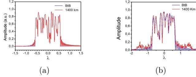
**Figure 3.13:** A relative error between the input and output in the nonlinear spectral amplitude  $\hat{q}(\lambda, \cdot)$  in (a) simulation, and (b) experiment for 16GHz NFDM transmissions.
