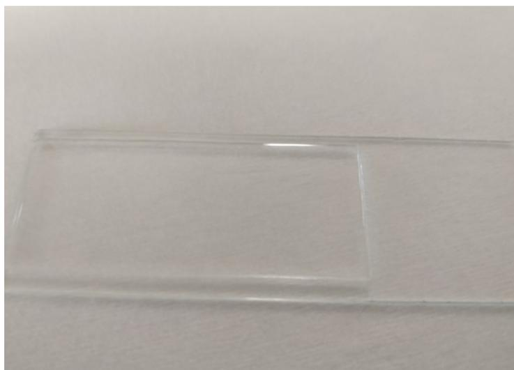
Figure 5.28 A PDMS stamp is on a common glass slide
