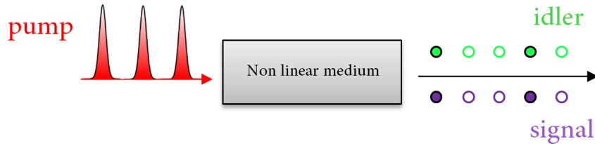
Fig. 1: Schematic describing a photon-pair source. The filled dots corresponds to photons whereas the empty dots corresponds to a non-generation (probabilistic process).
