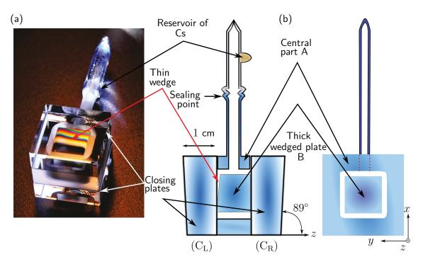
**Figure 5.2: Cell assembling** (a) Photograph of the cell. (b) Schematic of the cell (front view and side view).
