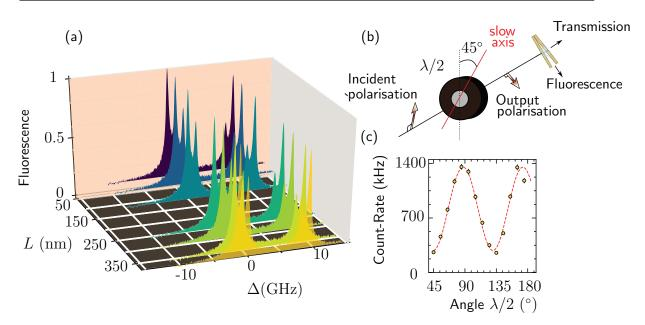
Figure 5.8: First fluorescence spectra (a)  $90^{\circ}$  off-axis fluorescence spectra obtained for  $\Theta = 220^{\circ}$ C and a range of thickness going from 50 nm (purple) to 376 nm (yellow). (b) Optimal configuration to reduce the stray light on the detector. The linear polarization after the half-wave plate needs to be in the direction of the detection path. (c) Count-rate on the SPCM as a function of the wave-plate angle.
