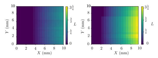
Figure 5.6: Wedge thickness characterization We have built two cells with different wedge angles. We represent the 2D mapping of the two wedges thickness (resolution of the prism along x and y axes: 0.5 mm)
