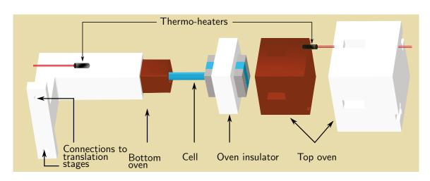
**Figure 5.4:** New oven design Thermo-heaters are introduced in copper via appropriated apertures in the Teflon parts. The two copper ovens are separated by a 1-cm PTFE piece. Connections to translation stages have been manufactured in order to have the possibility to move the cell with respect to the laser beam and hence probe different cell thicknesses.
