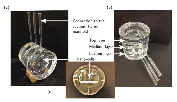
**Figure 5.1: The Big-mac** Photographs of the initial solution for the nano-cells project. The nano-cells are in the medium layer and the Newton colors (photograph (c)) indicate the varying in the cells thickness. The photographs are taken prior to filling with the alkali.
