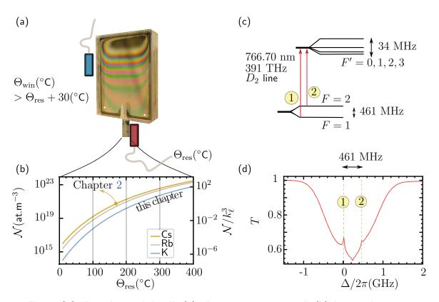
**Figure 3.2: Experimental details** (a) The potassium nano-cell. (b) Atomic density as a function of the reservoir temperature. (c) Energy diagram for the potassium  $D_2$  line. (d) Saturated absorption spectrum used for frequency calibration in a 7-cm potassium reference cell.
