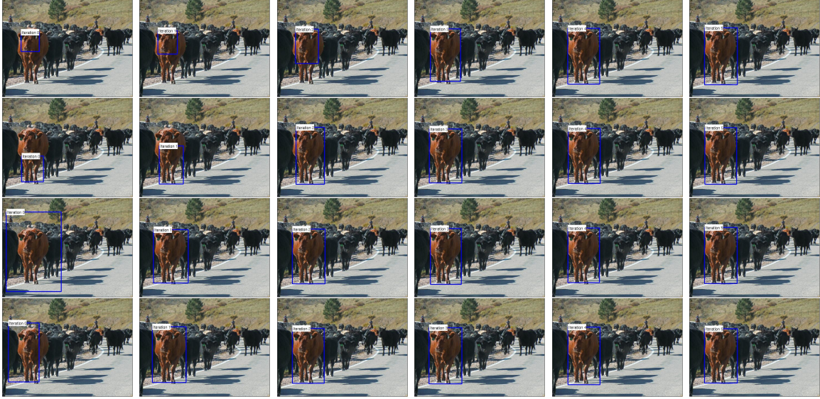
Figure 3-11: Illustration of the consecutive bounding box predictions made by our category agnostic location refinement module. In each row, from left to right we depict a seed box (iteration 0) and the bounding box predictions in each iteration. Despite the fact that the seed box might be quite far from the object (in terms of center location, scale and/or aspect ratio) the refinement module has no problem in converging to the bounding box closest to the seed box object. This capability is not affected even in the case that the seed box contains also other instances of the same category as in rows 3 and 4.
