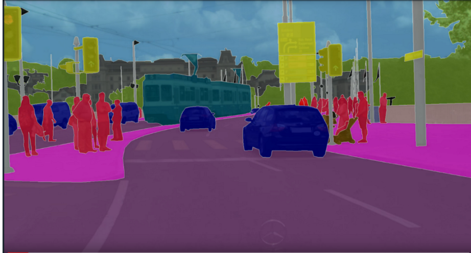
Figure 1-2: Pixel wise labeling - semantic segmentation example. We visualize the ground truth semantic label of each pixel of the image.
