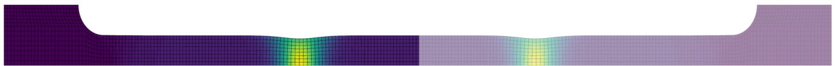
Figure 3.13: Plastic strain at end of computation for a very long tensile sample ( L/D = 32 ). Two necks emerged during the computation.
