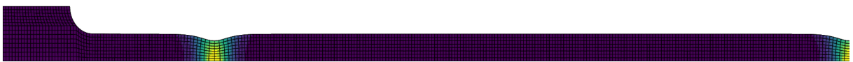
Figure 3.14: Double neck in half a sample for a very long tensile sample ( L/D = 12 ).
