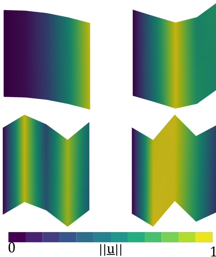
Figure 5.32: Eigen modes associated to the four vanishing eigenvalues in Figure 5.31. Any localization mode can be obtained as a linear combination of these four modes.
