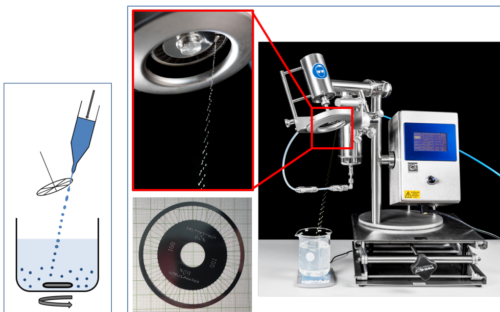
Figure 2.8 – Schematic representation (left) and pictures of the JetCutter (right) and one of the cutting tools used (bottom middle). Pictures provided by GeniaLab (Germany).
