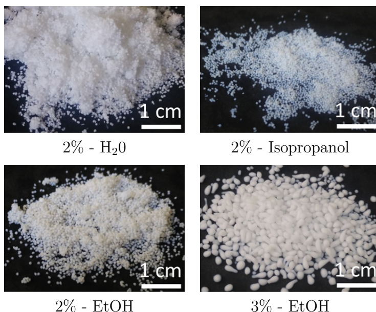
Figure 3.12 – Cellulose aerogel beads from various cellulose-[DBNH][Pr] solution concentrations and coagulation bathes. Adapted from Druel et al. (2018).
