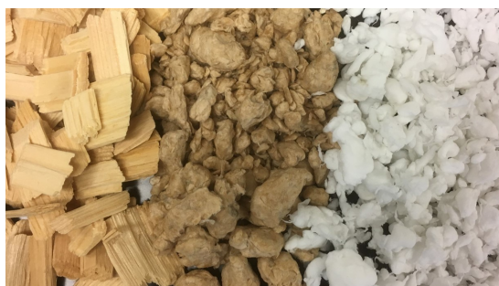
Figure 2.1 – Photo of the pulps after treatments: chips (left), unbleached pulp (middle) and bleached pulp (right). Photo taken by RISE-Innventia.
