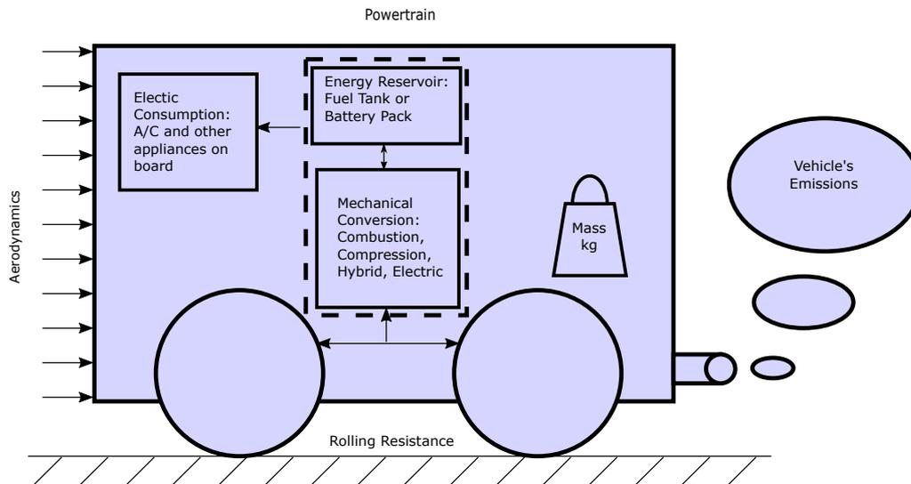
FIGURE 2.2 – Main low carbon technology bricks in a vehicle. Source: The Author.
