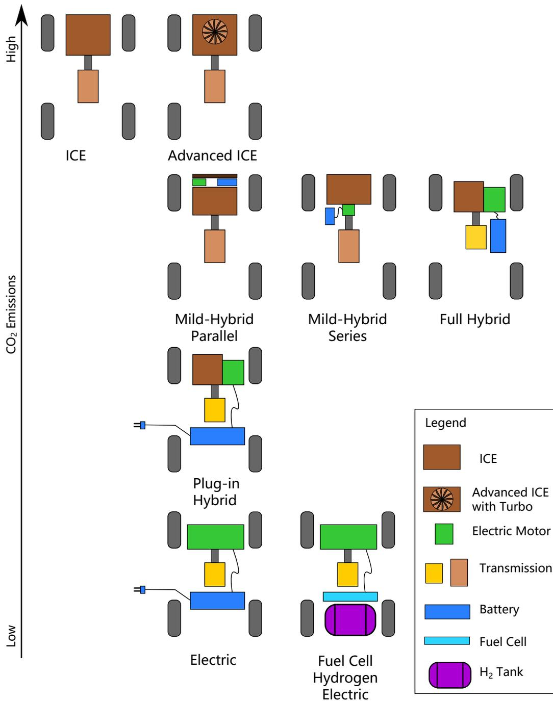
FIGURE 1.3 – Powertrain configuration of Automotive technologies to reduce CO<sub>2</sub> emissions. The CO<sub>2</sub> tail-pipe emissions order of each configuration is shown on the Y-axis. Source: The Author.
