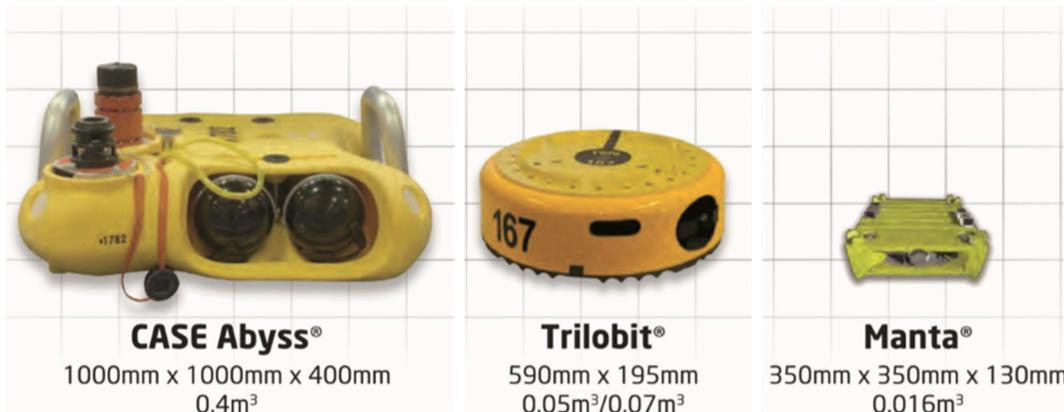
Figure 17: The evolution of deep-water nodes. Three deep-water ocean bottom nodes displayed to scale which have decreased in size over time, directly affecting ROV deployment efficiency. From [Bunting and Moses, \(2016\)](#).
