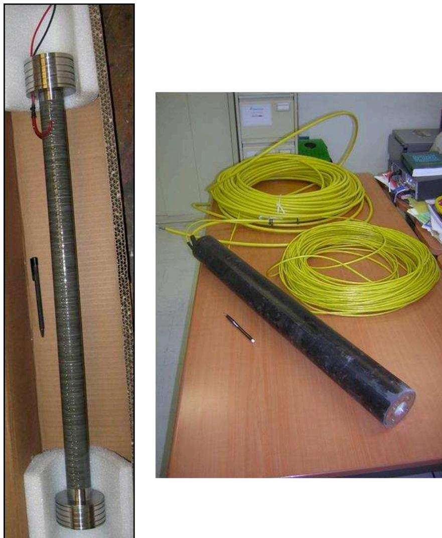
Figure 4: A typical piezo-actuator seismic source pillar without the polyurethane (left) and with the polyurethane envelope (right).
