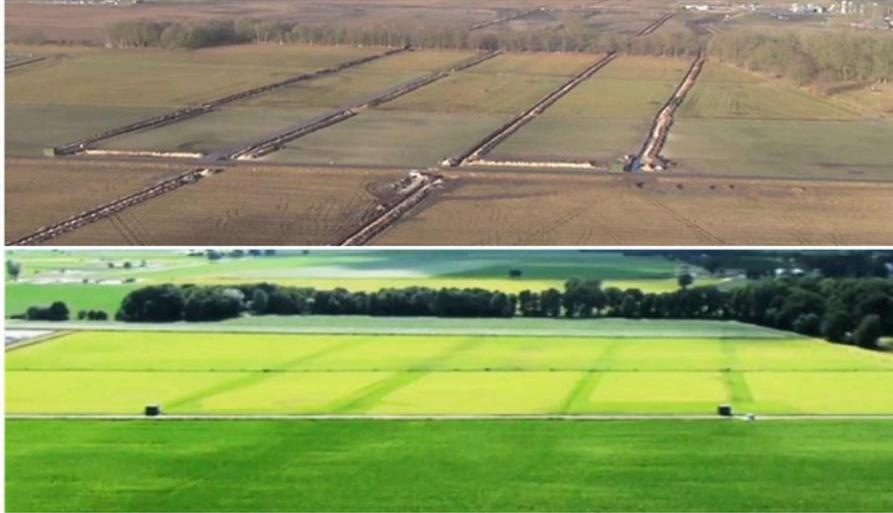
Figure 38: Aerial photos of the monitoring area. Top: Trenches during installation. Bottom: Four months later during continuous monitoring.
