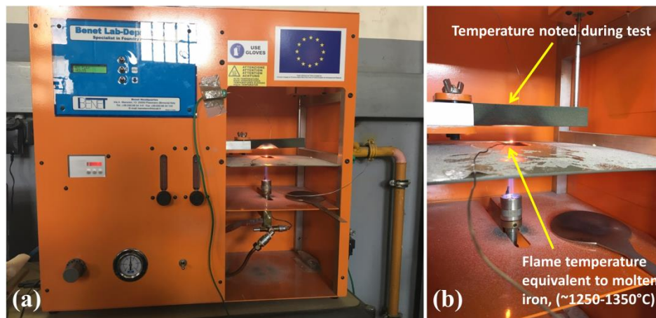
Figure 97. (a) Thermal deformation testing machine, and (b) zoomed view
