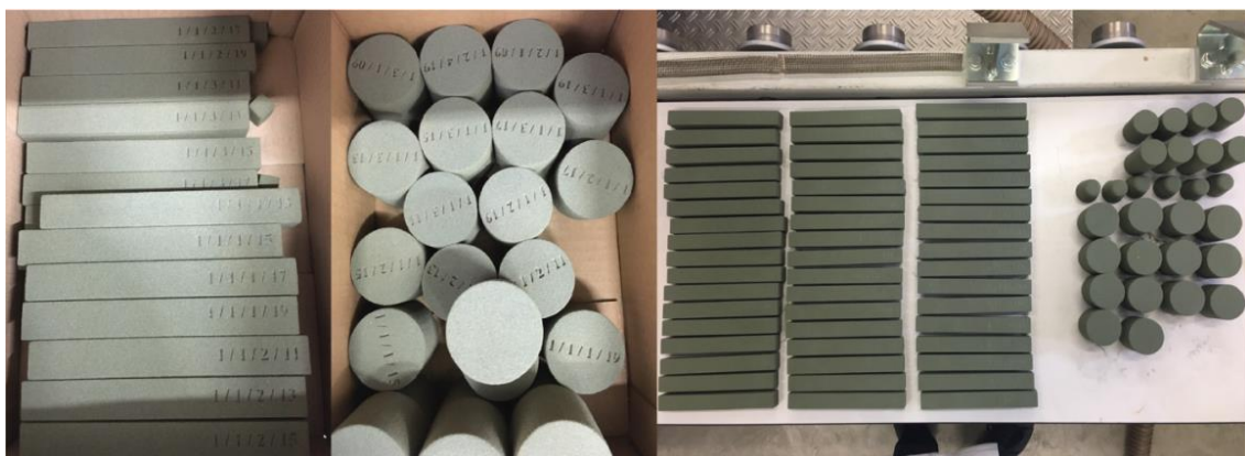
Figure 24. 3D printed 3PB test bars and permeability specimens
