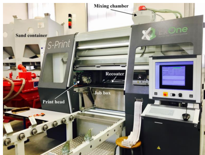
Figure 22. 3D sand printer used in the present experiments
