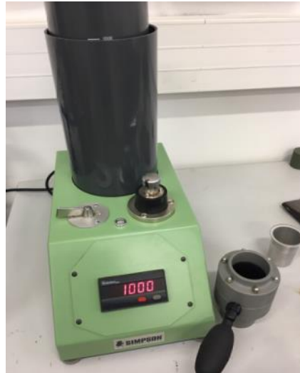
Figure 31. Universal machine used for the gas permeability test[79]
