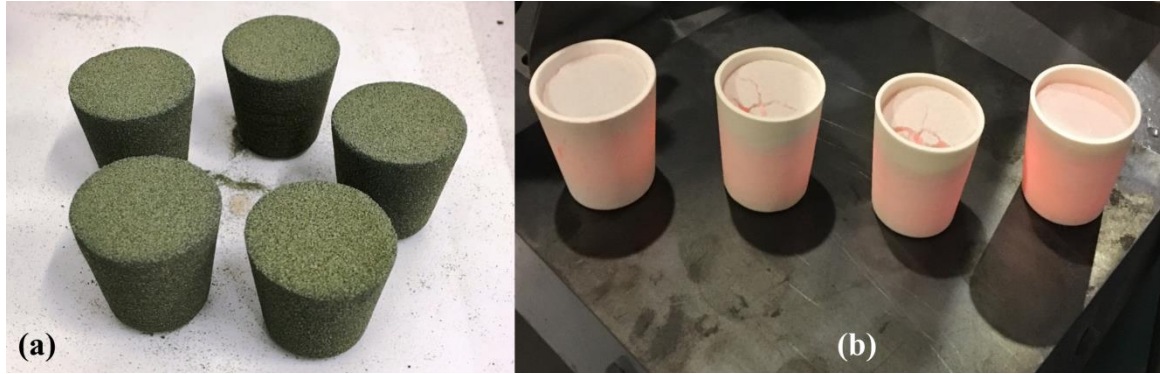
Figure 43. LOI test (a) 3DP samples, (b) immediately after taking out of the oven at 900 °C
