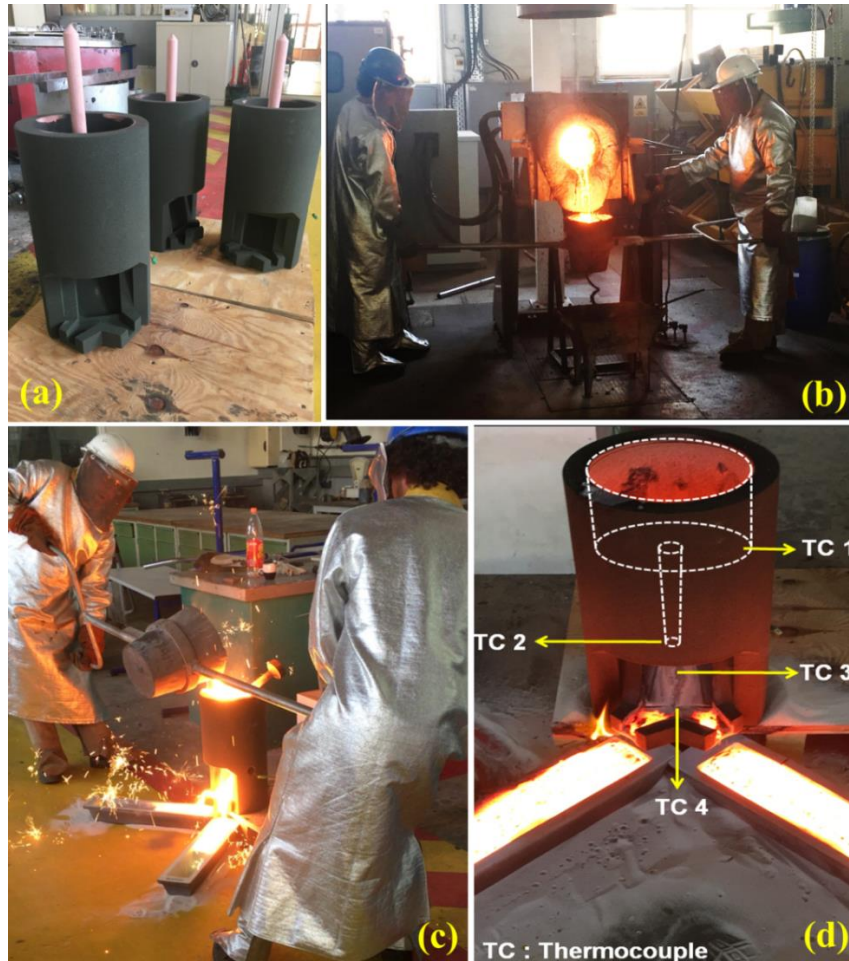
Figure 94. Steps involved, (a) 3D printing of sand mold, (b) melting iron, (c) casting process and (d) eroded molded with the respective positioning of thermocouples.
