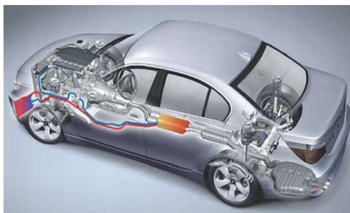
Fig. 1.32: BMW series 5 with TEG as waste heat recovery system [TE101]
