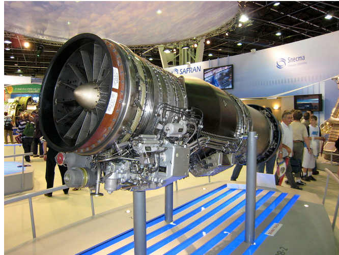
Figure 1.1: Gas turbine engine (Safran M88-2, manufactured by Safran Aircraft Engines) which has components subjected to complex loadings 1
