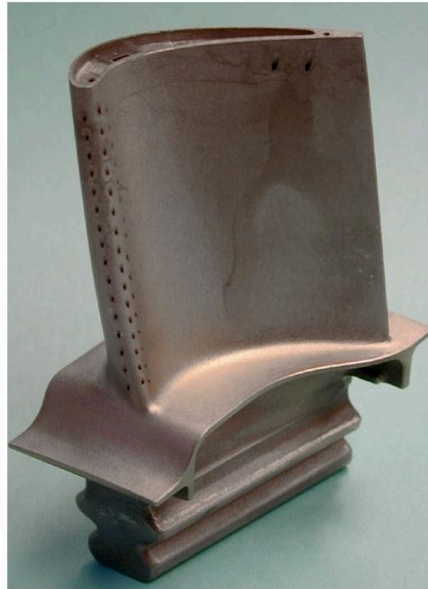
Figure 1.2: High pressure turbine blade which is usually the limiting component of a jet engine
