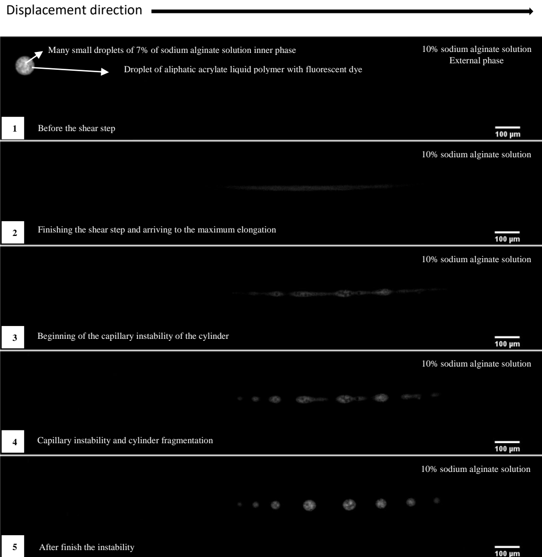
Figure 4-1-A 1 Fragmentation of double emulsion with low viscosity ratio \eta_1/\eta_2 = 0.28
