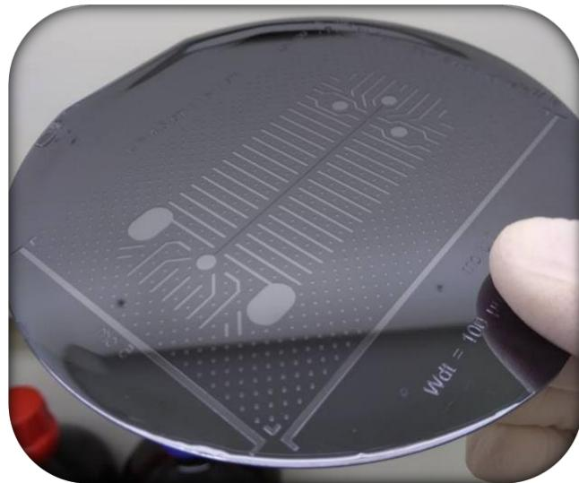
**Figure 5 – Silicon wafer with SU8 deposit for the fabrication of a cross-shaped microsystem**
