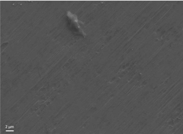
Figure 3.1 SEM surface morphology of a 150µm thick Mo foil
