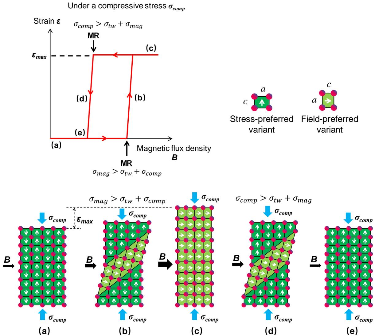
Figure 1.5 Schematic of magneto-mechanical loading-induced reversible martensite reorientation.
