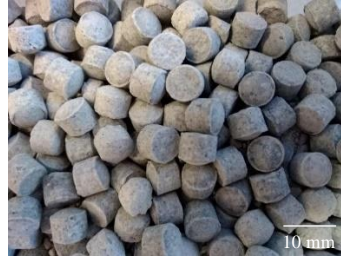
Figure 3-2: Assembly of the MX80 pellets used in the present work.
