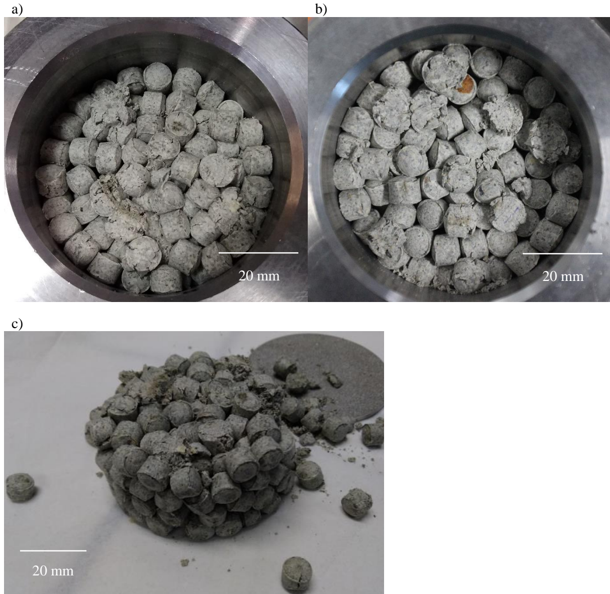
Figure 3-16: Picture of samples SP0a and SP0b after dismantling. a: SP0a equilibrated at 9 MPa of suction; b: SP0b equilibrated at 4 MPa of suction; c: SP0a removed from the isochoric cell.
