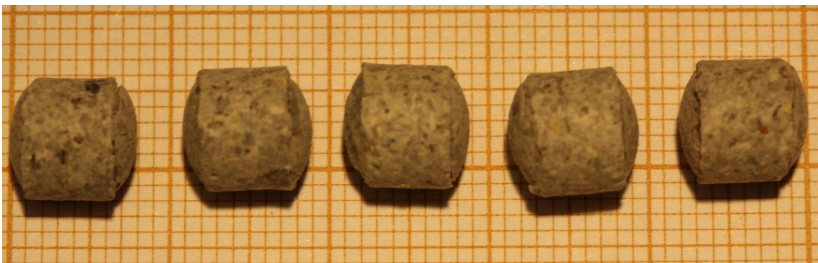
Figure 4-14: Picture of 7-mm pellets at equilibrium at 9 MPa suction.
