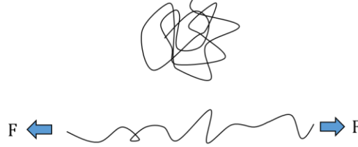
Figure 5 Illustration of the change in entropy for the large deformation of elastomers
