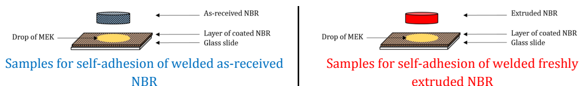
Figure 21 Illustration of the two systems: self-adhesion of welded as-received (blue) and freshly extruded (red) NBR
