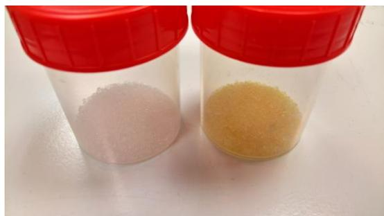
Figure 4-23. The photo of silica aerogel support before and after plasma experiments.
