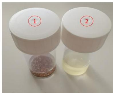
Figure 5-22. Photo of spent samples (2 h) in pure acetone: 1). HZSM-5, 2). SiO<sub>2</sub> aerogel.
