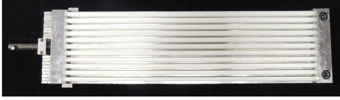
Figure 3.1: Mold used for cement pastes preparations. The mold may give up to 10 samples of dimensions 300 mm×13 mm×3 mm.
