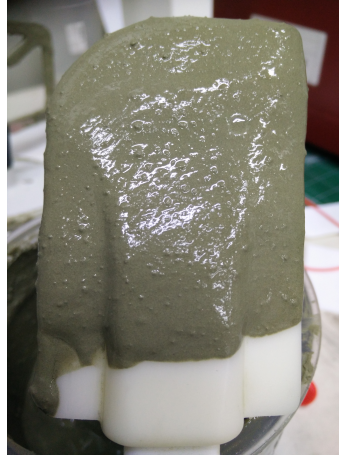
Figure A.1: Formed lumps during mixing of pastes at high alkali content and in presence of SRA.
