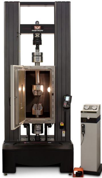
FIGURE 2.12: Tensile tests setup: Instron machine ref 5980
