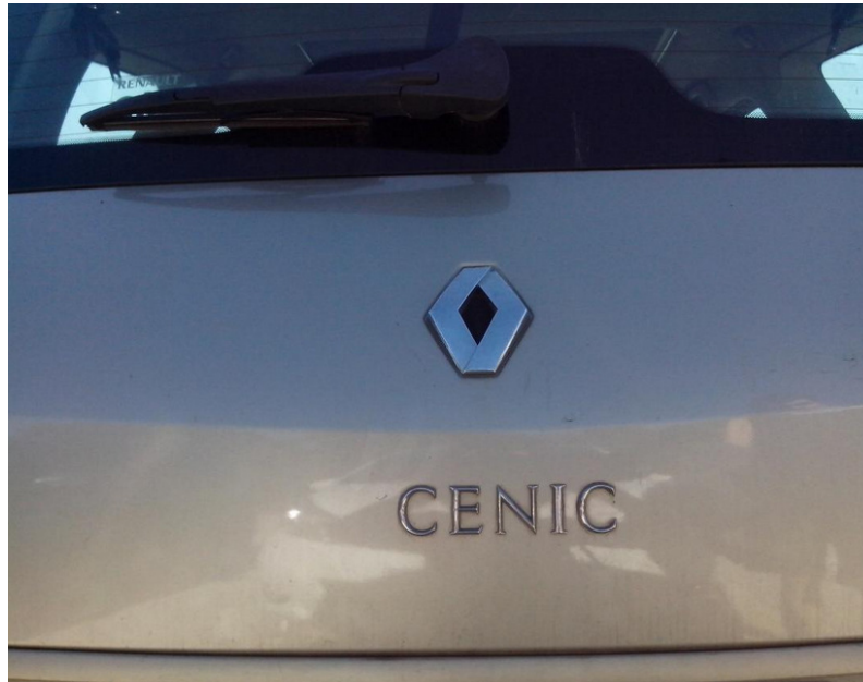
FIGURE 1.2: Letters debonding on the trunk of a car
