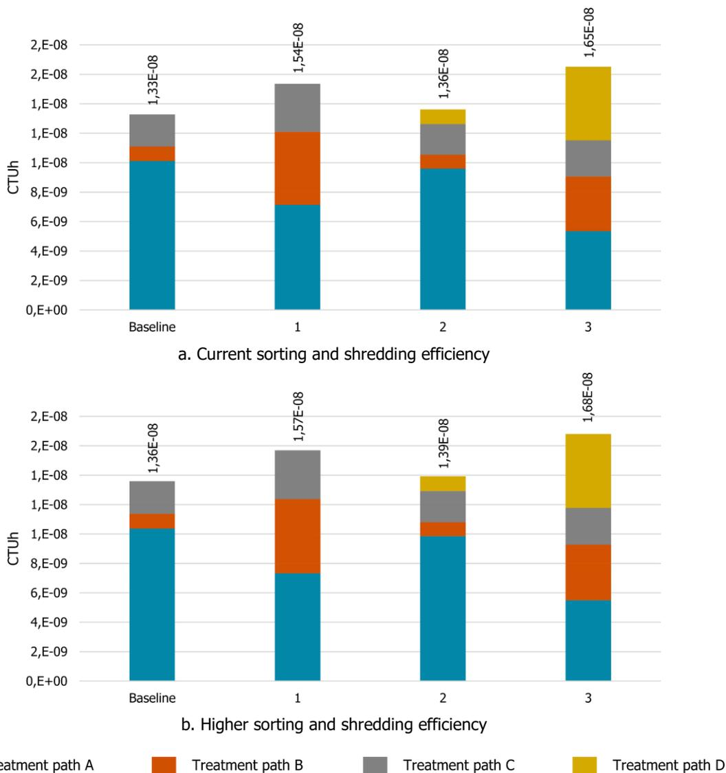
Figure 5-4. Sensitivity analysis of tablets treatment scenarios: human toxicity potential.
