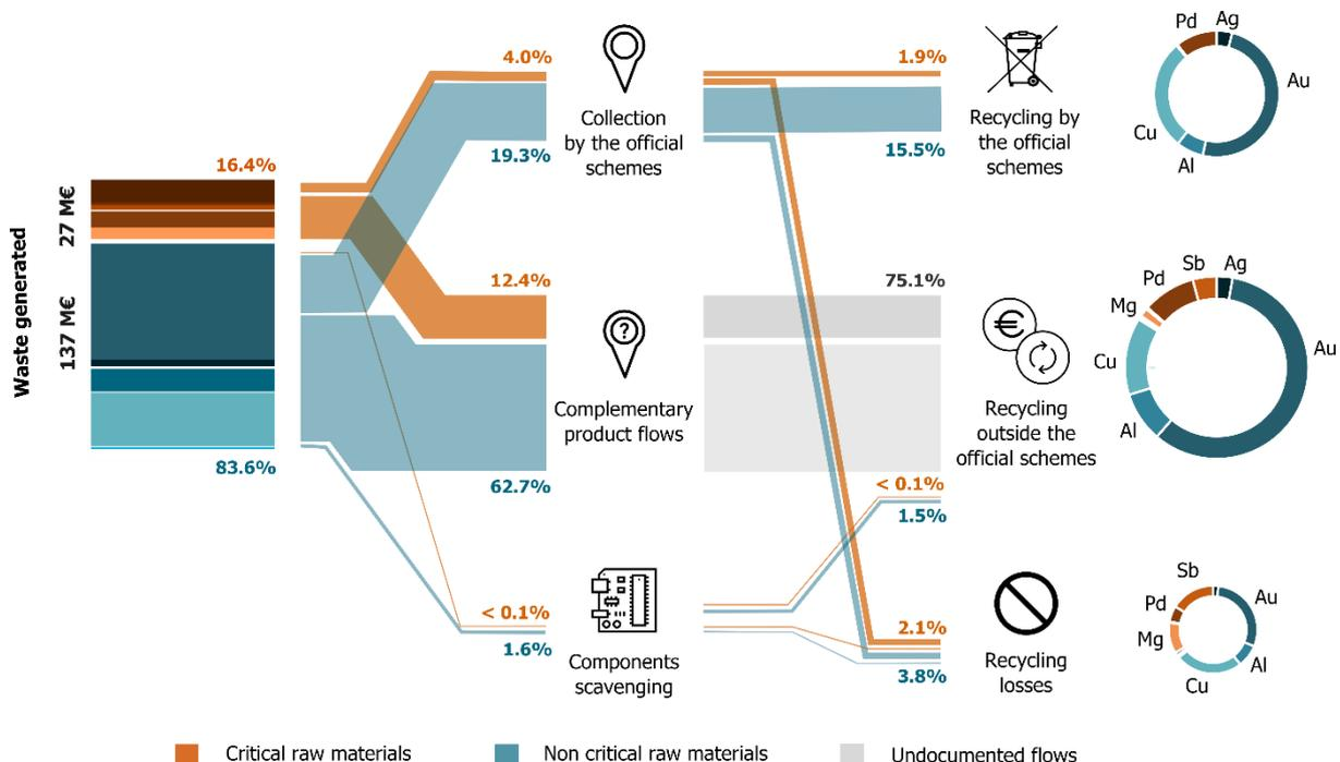
Figure 8-7. WEEE screens flows: target materials generated, collected and recycled (economic-based approach).
