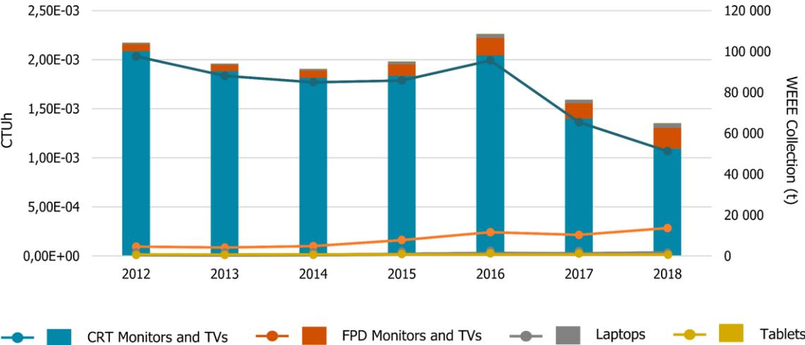
Figure 5-11. Total toxicity impacts for treating screens collected in France from 2012 to 2018.
