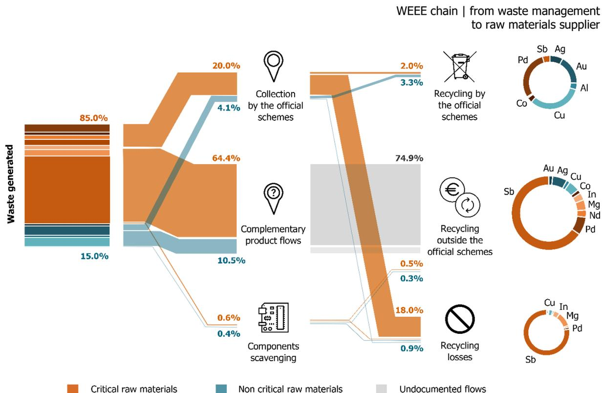
Figure 8-9. WEEE screens flows: target materials generated, collected and recycled (criticality weighted-based approach).
