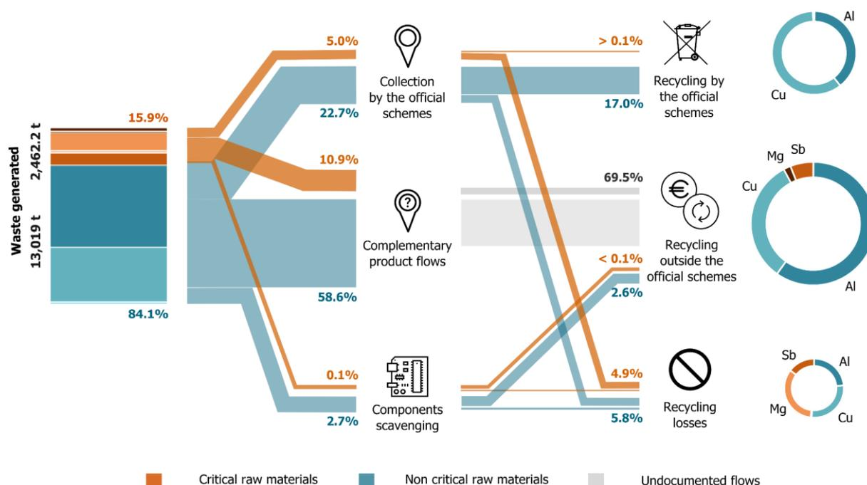
Figure 8-3. WEEE screens flows: target materials generated, collected and recycled (weight-based approach).
