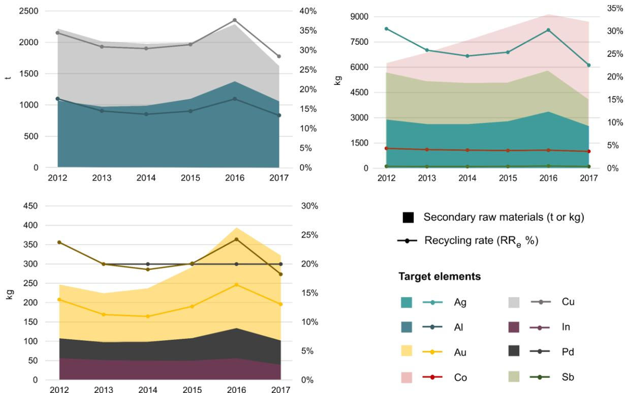
Figure 4-21. Recycling rate of target elements (RR<sub>e</sub>) in WEEE category II (2012-2017).
