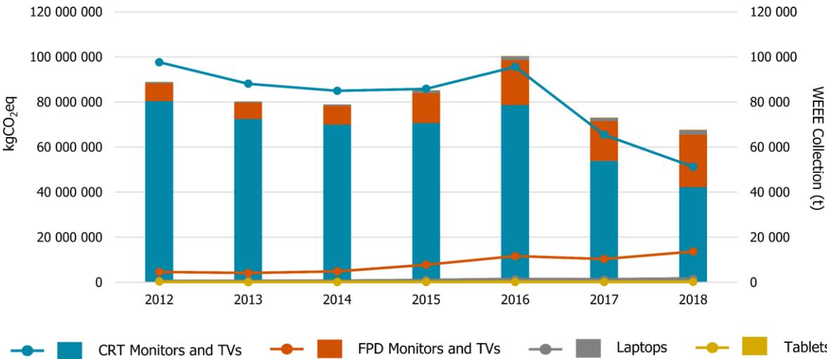
Figure 5-10. Total potential global warming impacts from treating screens collected in France from 2012 to 2018.
