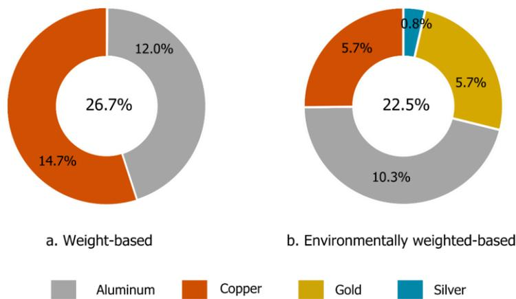
Figure 5-15. Treatment rate of aluminum, copper, gold, silver in FPD screens in France: comparison of two approaches.
