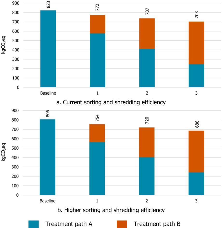
Figure 5-8. Sensitivity analysis of CRT monitors and TVs treatment scenarios: global warming potential.
