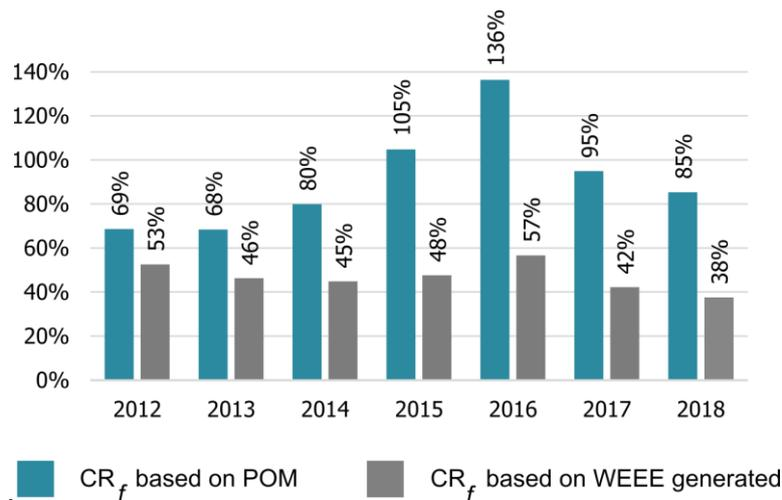
Figure 4-10. Comparison of different approaches for calculating WEEE category II collection rate.
