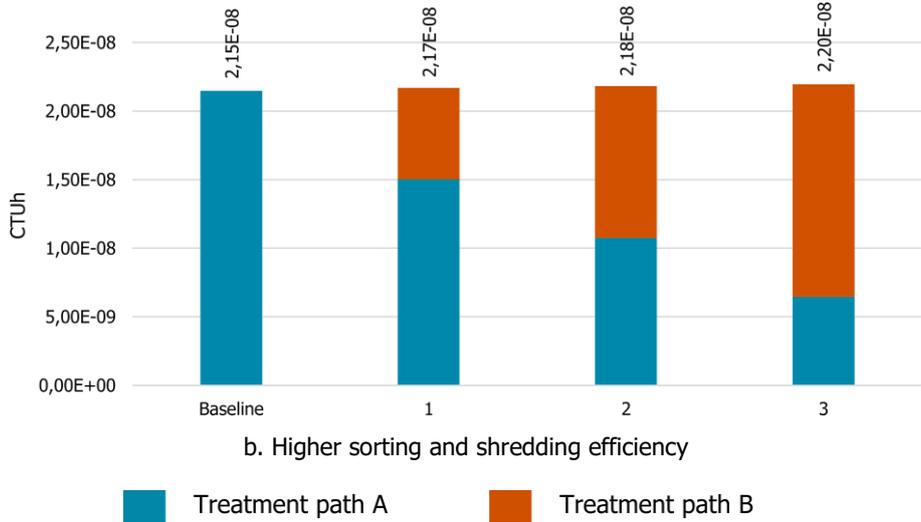
Figure 5-9. Sensitivity analysis of CRT monitors and TVs treatment scenarios: human toxicity potential.
