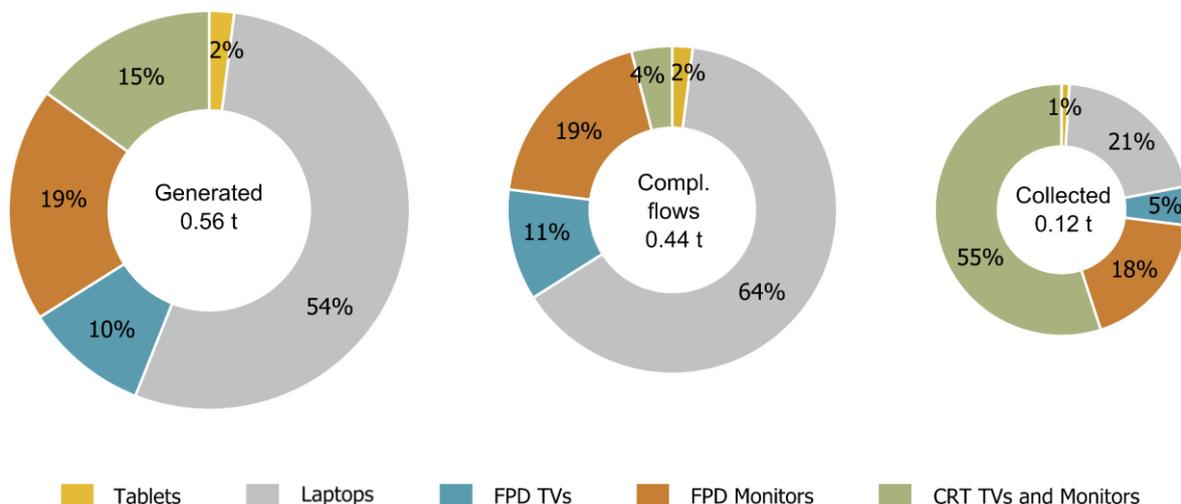
Figure 4-13. Total weight and share of palladium per UNU-keys in screens in France (2017).
