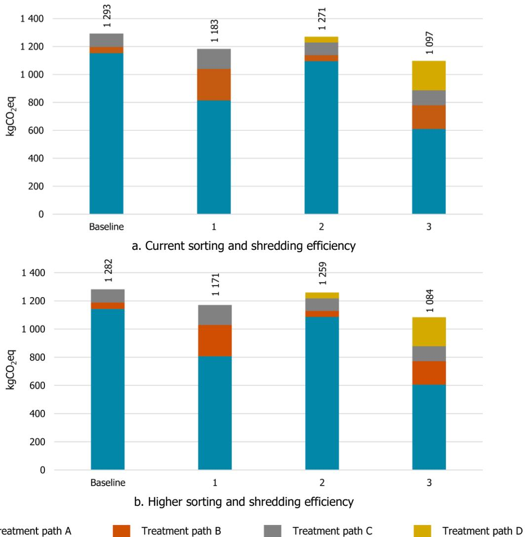
Figure 5-3. Sensitivity analysis of tablets treatment scenarios: global warming potential.
