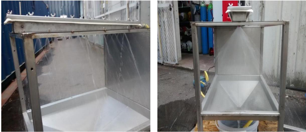
*Figure 1.13: A picture of the proposed system with the spraying desiccant*
