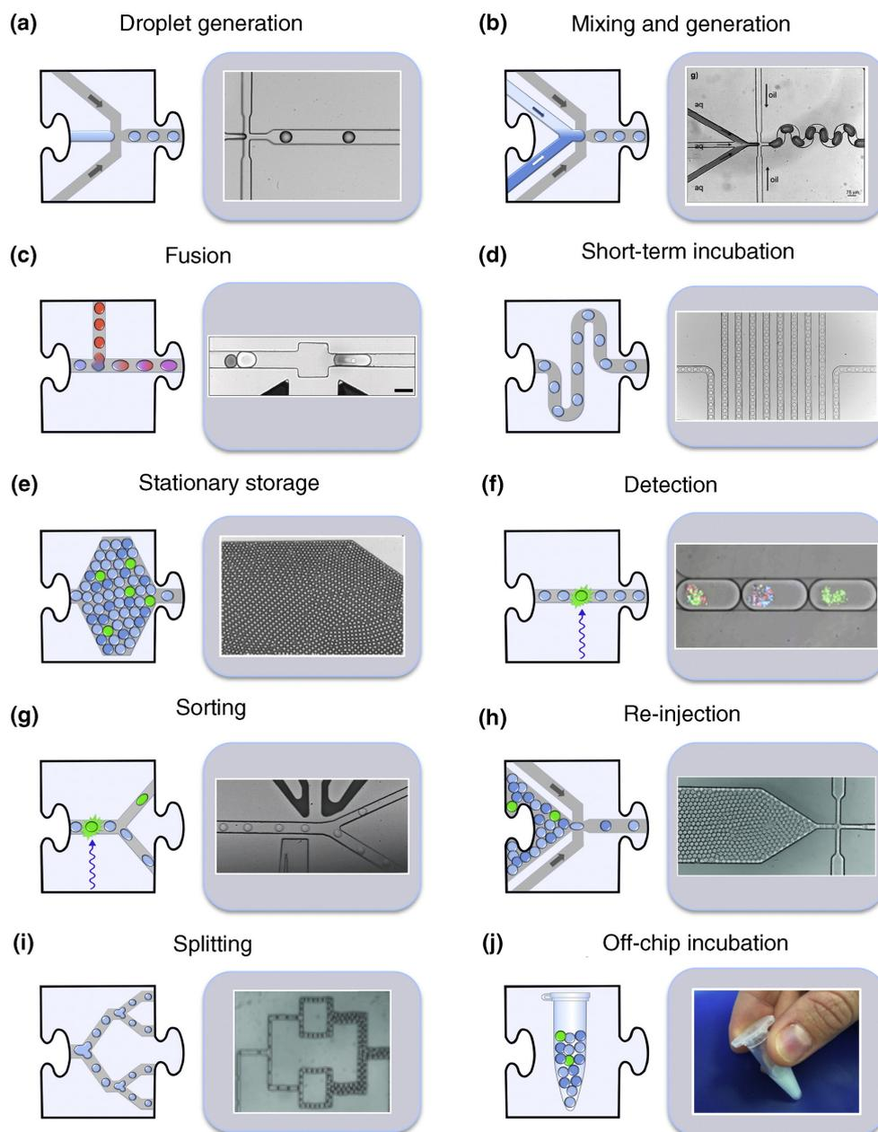
Figure 2.2.1: **Examples of microfluidic modules for manipulating droplets.**
