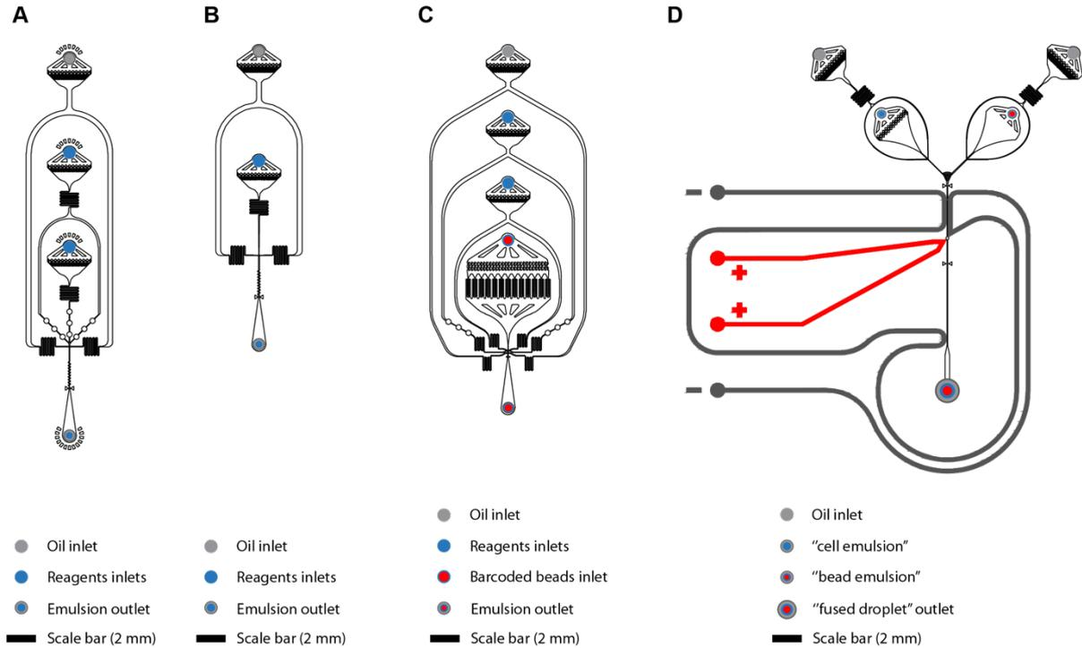
**Fig. S2. Design of microfluidic devices.** (A) Device used to compartmentalize cells in 45 pl droplets. (B) Device used to produce 9 pl droplets to make hydrogel beads. (C) Device used for compartmentalization of hydrogel beads in 100 pl droplets. (D) Device used to merge nucleosome-containing droplets with hydrogel barcoded bead-containing droplets. Potential and ground electrodes are indicated with the '+' and the '-' marks, respectively. Scale bars are 2 mm.
