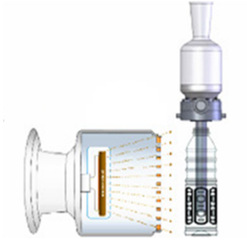
Figure 2.6: Bottle sterilisation by electron-beam irradiation.
