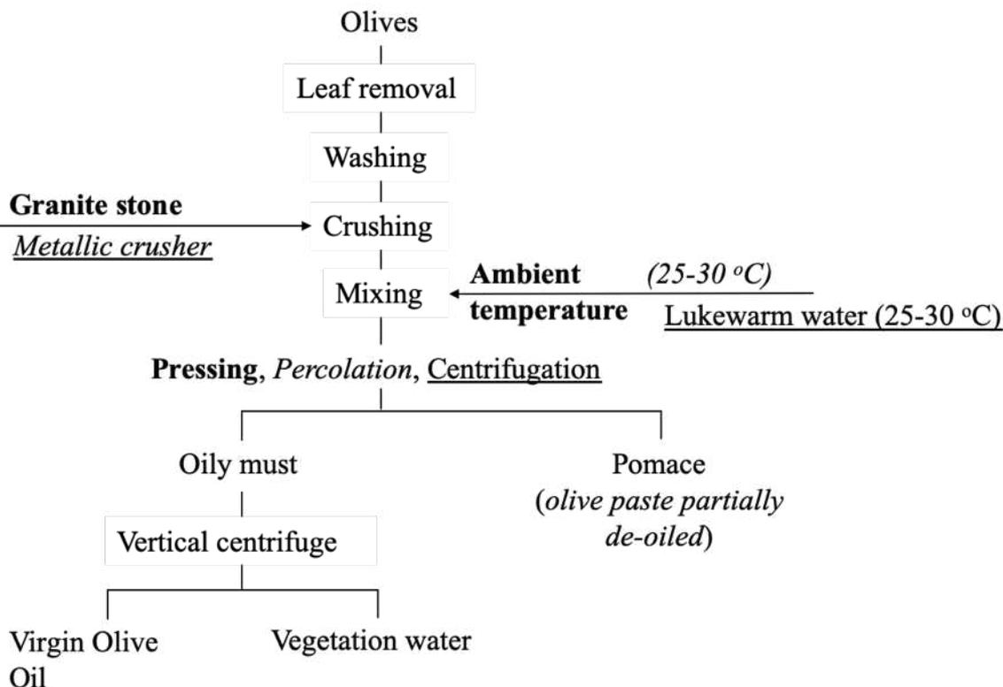
Figure 6. Diagram of olive oil extraction by different mechanical techniques (Giovacchino, 2000)
