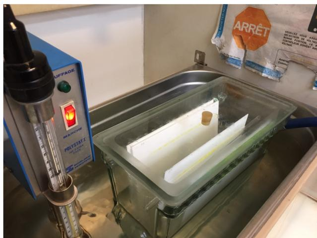
*Figure 19. Developing chamber for TLC plates*
