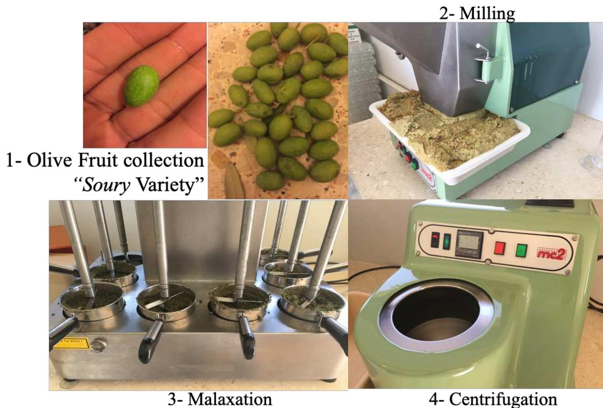
Figure 14. Olive oil extraction process
