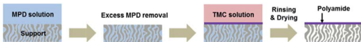
Figure 1.1: Schematic illustration of the fabrication of APA TFC membranes via conventional IP, from Park et al. , (2017)[94].
