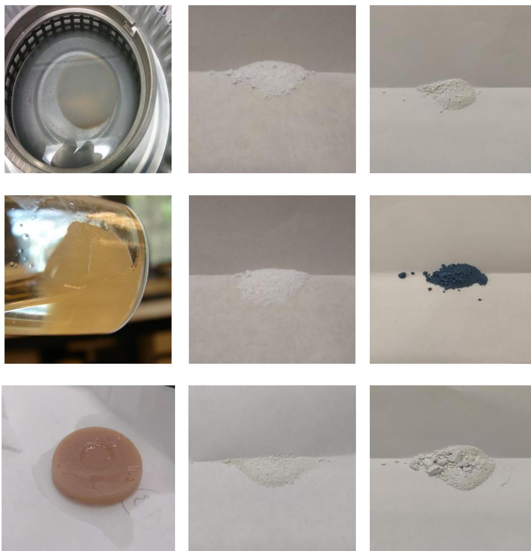
**Figure 3.5** Same sequence for each material: TO on the top, ATO in the centre and TaTO at the bottom. From left to right: image of the gel, image of the amorphous aerogel after drying with SC  $\text{CO}_2$ , and image of the calcined aerogel.
