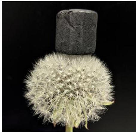
**Figure 1.27** Image of a graphene aerogel illustrating the low density of the material.<sup>151</sup>
