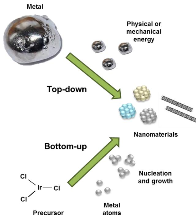
Figure 1.24 Bottom-up and top-down approaches to nanomaterials construction.
