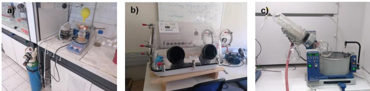
**Figure 3.1** (a) Reactor flask under Argon atmosphere. The reactor flask is connected to a balloon filled with the inert gas in order to maintain the Ar atmosphere; (b) the glove box under inert atmosphere (Argon) where some procedures, as filtrations, were taken place; (c) the rotatory evaporator, used for evaporating the solvent and by-products of the synthesis from the desired product.
