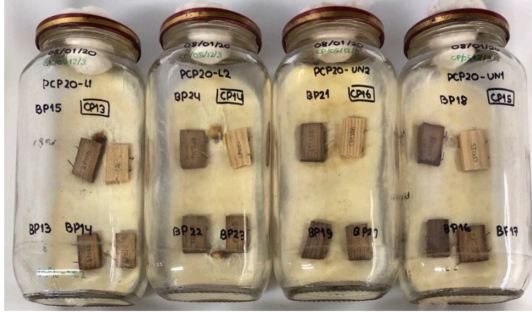
Figure 8.6: Fungal test device with wood specimens
