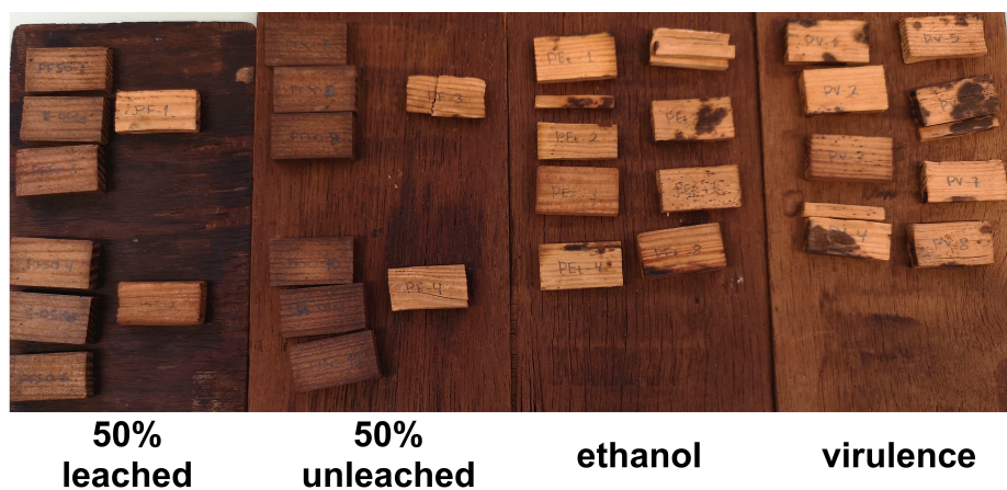
Figure 9.22: Pine samples at the end of decay test (exposed to C. puteana )
