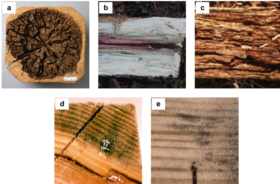
Figure 2.2: Attack of fungi on wood: a) brown-rot (Goodell, 2020); b) white-rot (Auró 2016); c) soft-rot (Mariano et al., 2020); d) blue stain (Goodell, 2020); and e) mold (Imken et al., 2020)
