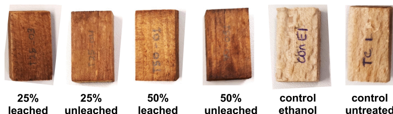
Figure 9.25: Beech wood samples treated with different concentration of pyrolysis liquid at the end of the termites' test
