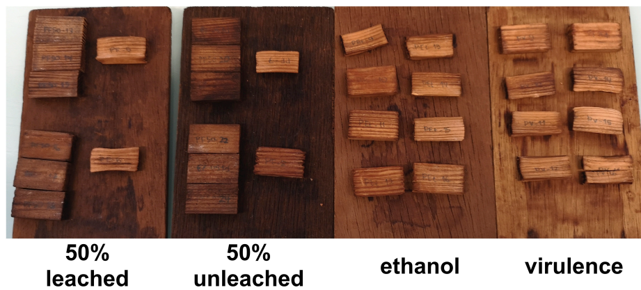
Figure 9.24: Pine samples at the end of decay test (exposed to R. placenta )
