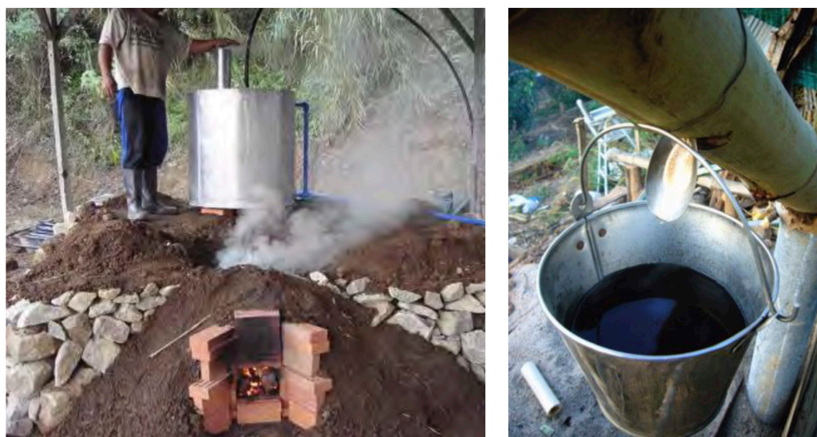
Figure 2.4: Traditional charcoal making process (left) and its by-product from the condensation of smoke (right) ( Kishimoto and Tsuyoshi, 2015 )
