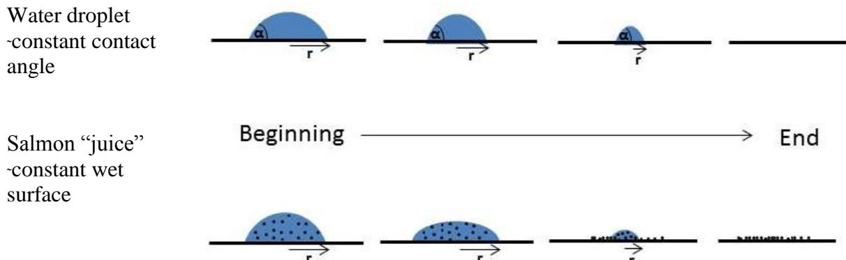
Figure 5: Two different mechanisms of wet surface evolution during drying of a droplet of water and salmon “juice”.
