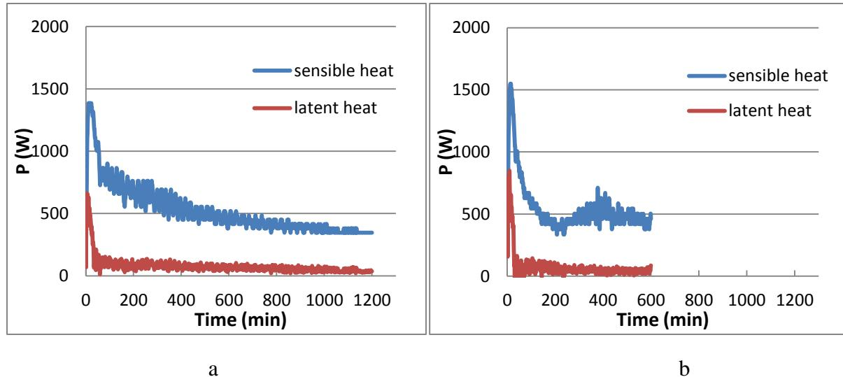
Figure 8: Evolution of the latent and sensible heat power during drying of 3 kg of water,
