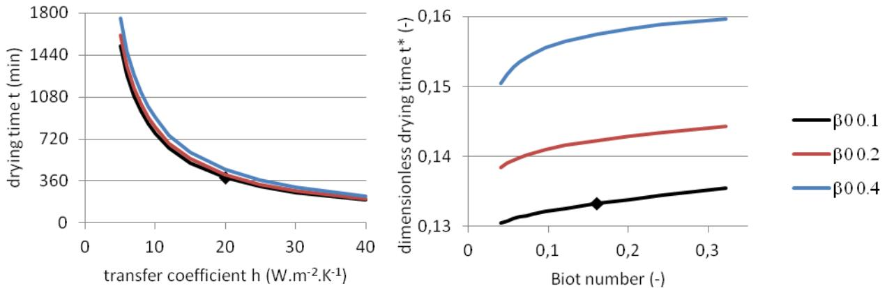
Fig. 13. Influence of heat transfer coefficient/Biot number on drying time
