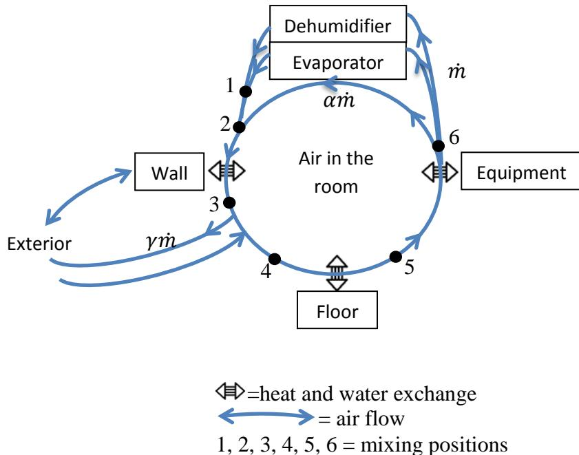
Figure 9: Scheme of the developed zonal model
