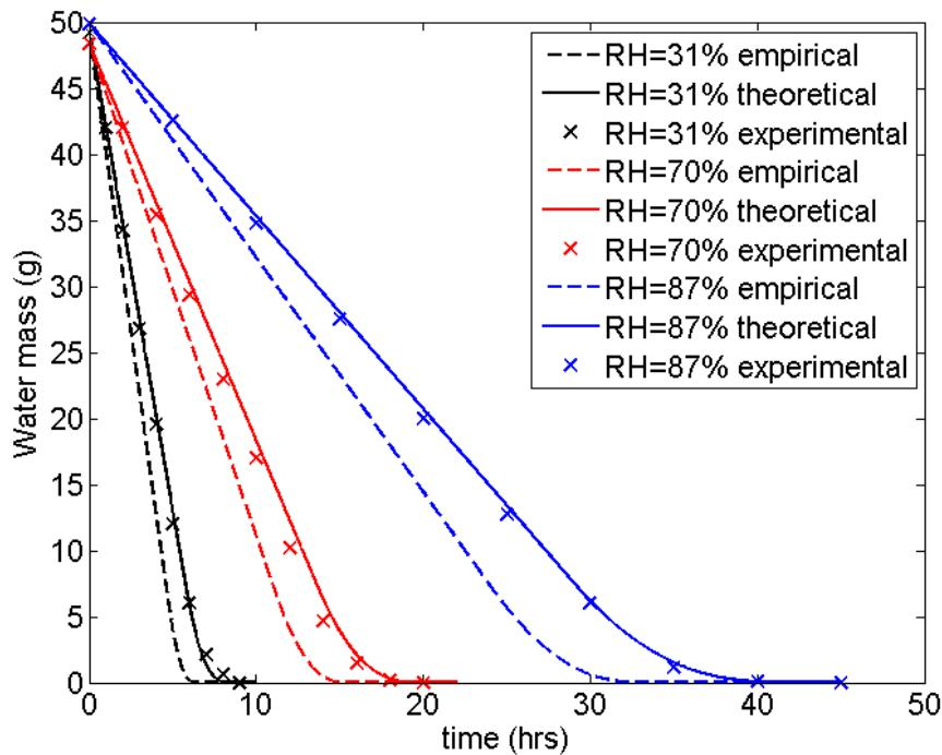
Figure 5: Water mass evolution during evaporation (2 periods): comparison between empirical model, theoretical model and experimental data.
