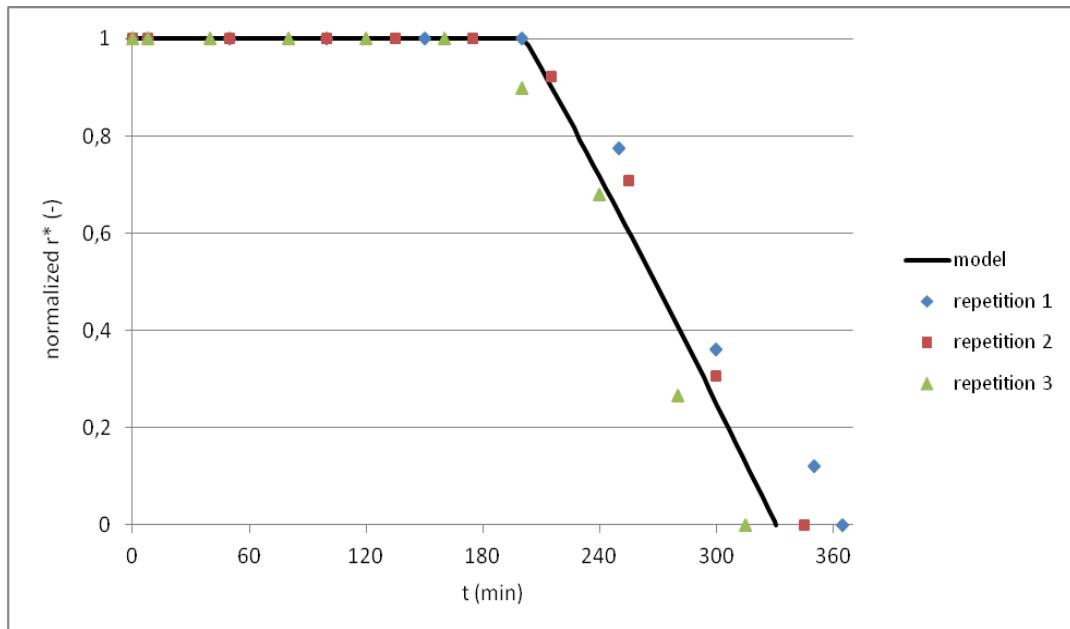
Fig. 5. Base radius evolution on stainless steel plate ( $r^* = r(t)/r_0$ ).
