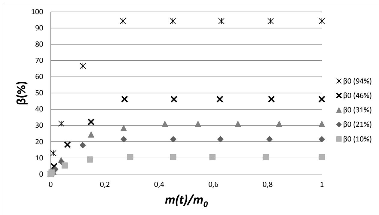
Figure 10: Evolution of the wet surface over the total surface ( $\beta$ ) in function of the water mass. Experiments performed inside a wind tunnel with different initial values of  $\beta_0$ : 10, 21, 31, 46 and 94% (4.2°C, 51% air relative humidity and 1.0 m.s<sup>-1</sup>)
