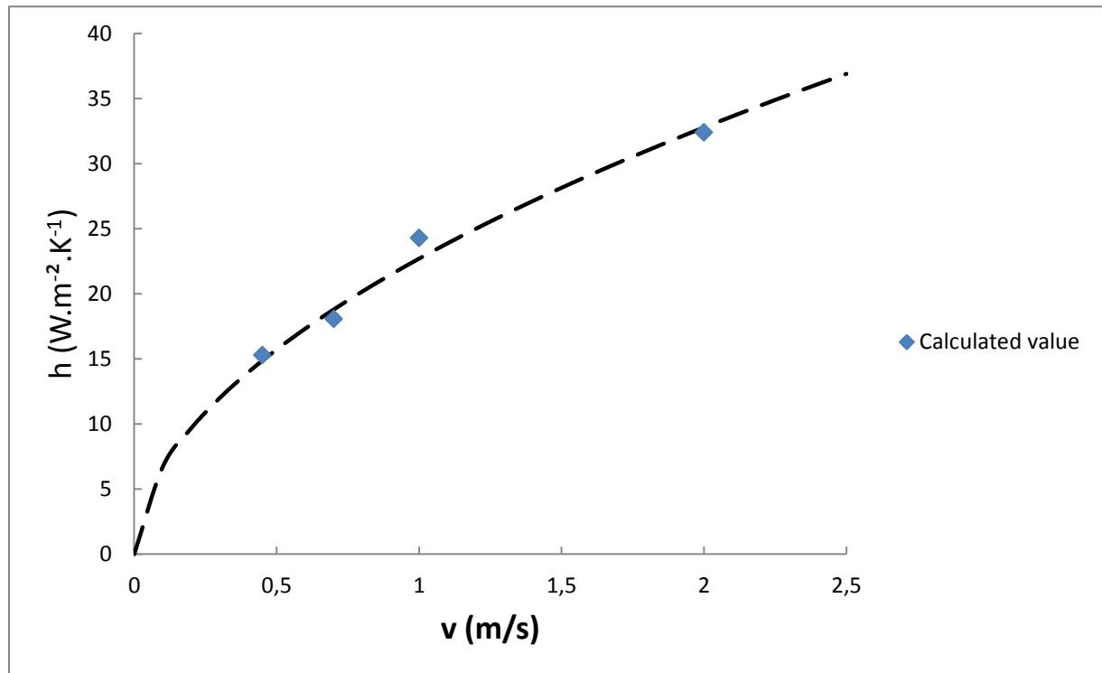
The heat transfer coefficient is almost proportional to the square root of the velocity, which corresponds to the expected laminar boundary layer: the maximal Reynolds number relative to the development of the hydrodynamic boundary layer along a plate (length,  $L = 0.15$  m) for an air velocity  $V$  of  $2.0 \text{ m.s}^{-1}$  is  $Re = \frac{V \cdot L}{\nu} \approx 2.10^4$ . This value is less than  $5.10^5$ , which is considered as the beginning of the turbulent boundary layer [30].
