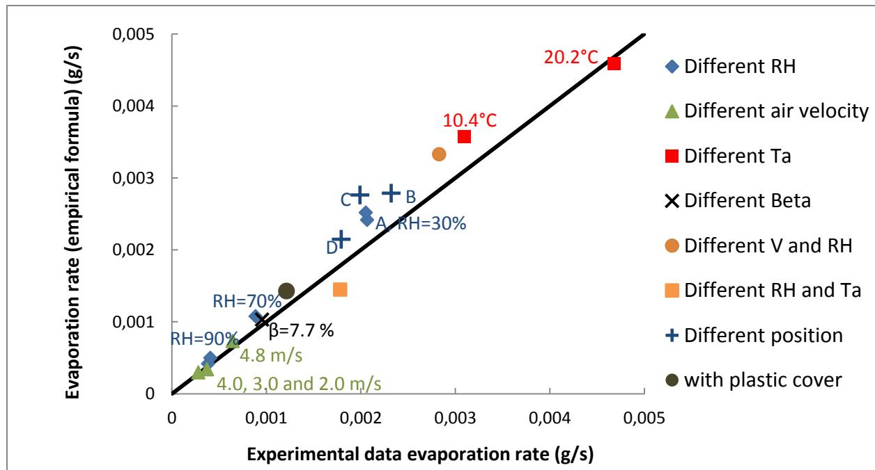
Figure 3: Evaporation rate comparison (1<sup>st</sup> period) between the experimental data and the empirical model
