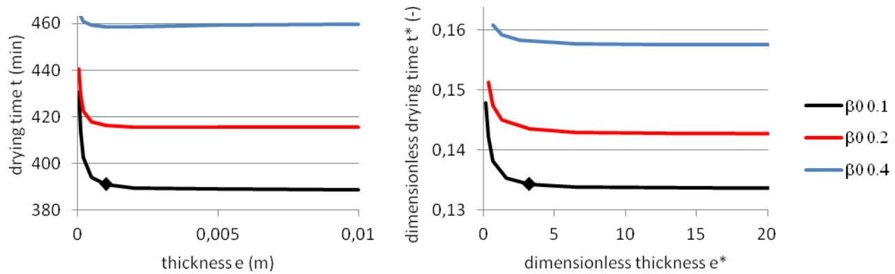
Fig. 12. Drying time versus plate thickness (dimensional /dimensionless)
