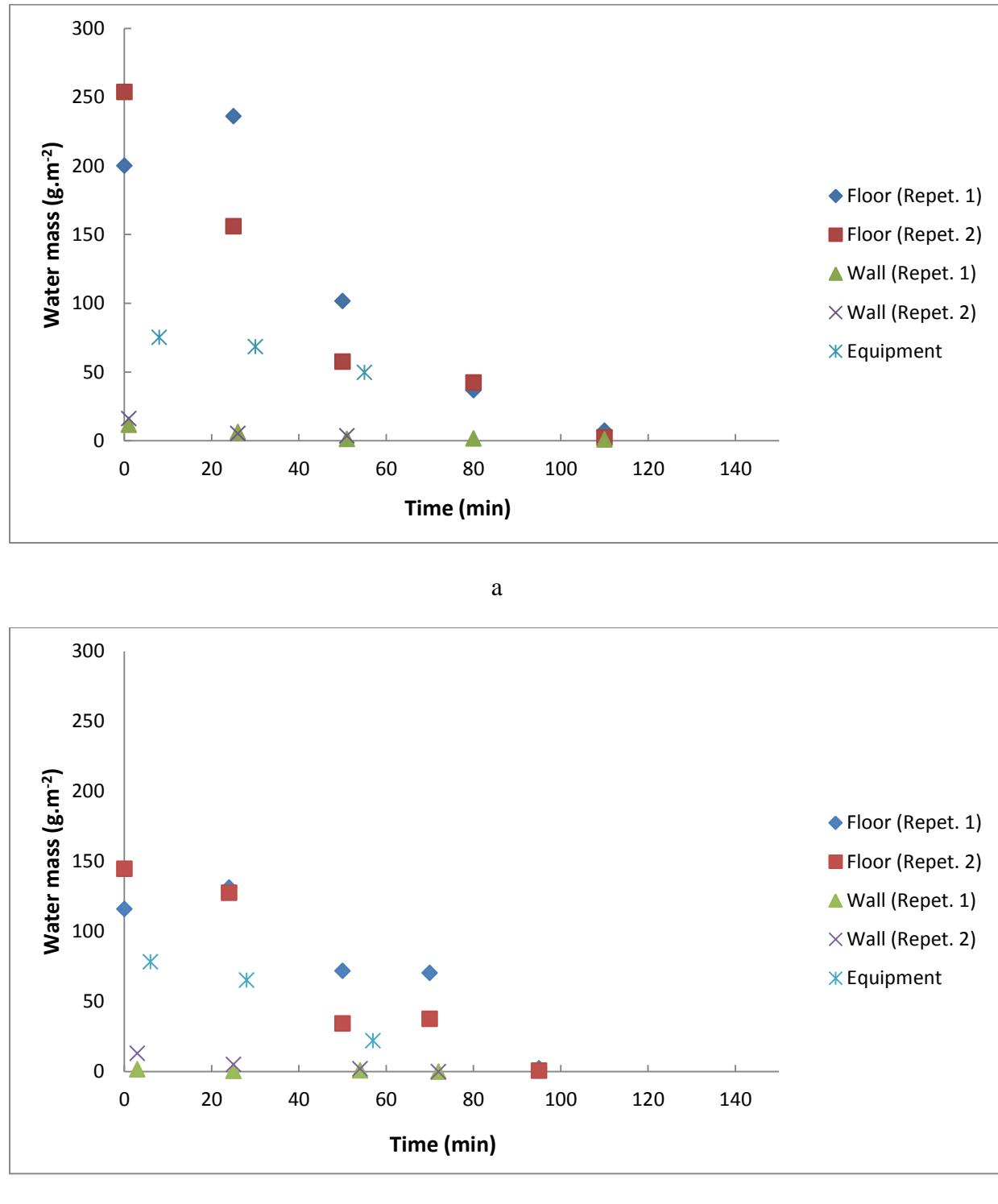
Figure 8: Water mass evolution on the wall, floor and equipment a- without a dehumidifier b- with a dehumidifier
