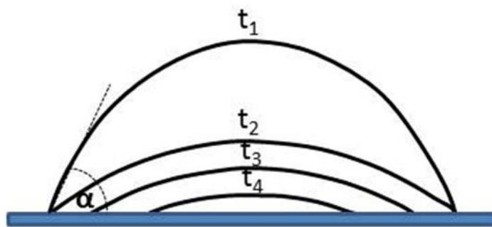
Figure 1: Droplet shape evolution during evaporation.
