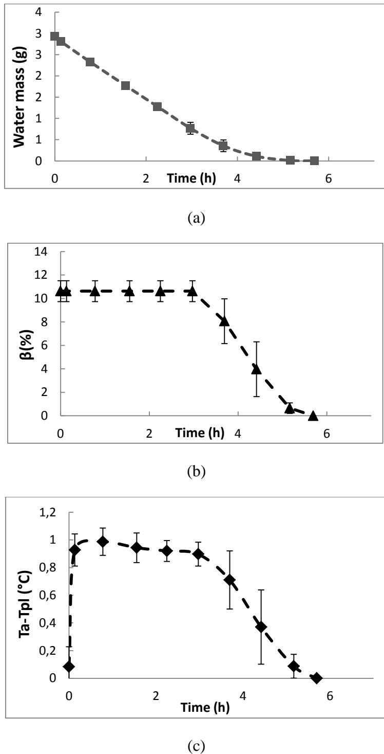
Figure 5: Influence on the evaporation rate of (a)-the air relative humidity (for experimental conditions of  $4.2^{\circ}\text{C}$ ,  $1.0 \text{ m.s}^{-1}$  and  $\beta_0\sim 10\%$ ) (b)-the air temperature (for experimental conditions of  $51\%RH$ ,  $1.0 \text{ m.s}^{-1}$ ,  $\beta_0\sim 10\%$ ) (c)-the air velocity (for experimental conditions of  $4.2^{\circ}\text{C}$ ,  $51\%RH$ ,  $\beta_0\sim 10\%$ )
