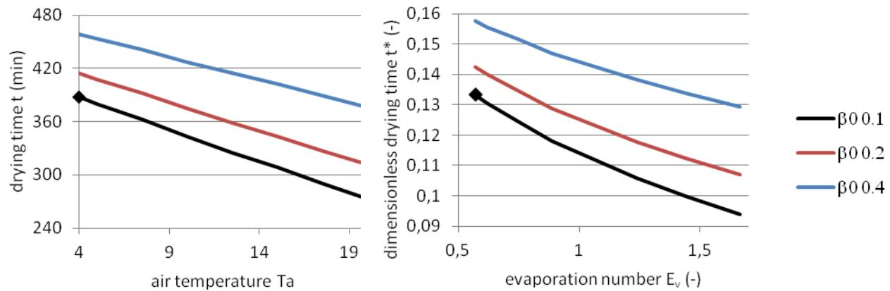
Fig. 15. Influence of air temperature/evaporation number on drying time
