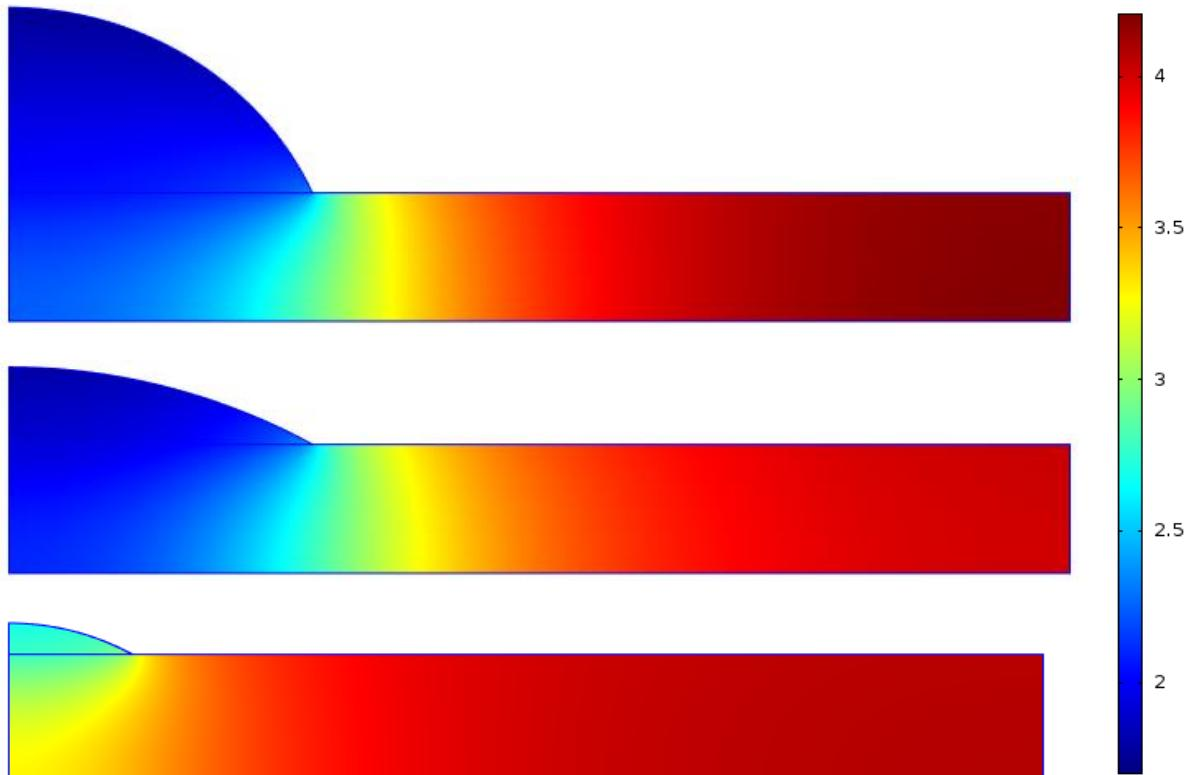
Fig. 11. Temperature field after 7 min, 220 min (end of the pinning period) and 460 min.
