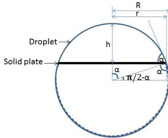
Figure 9: Side view of a droplet with the height “h” and the contact angle “ $\alpha$ ” on a solid plate.
