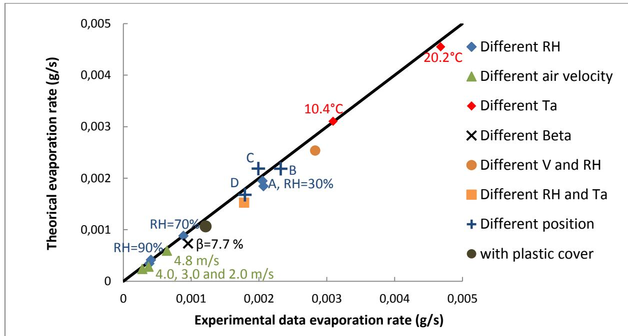
Figure 4: Evaporation rate comparison (1<sup>st</sup> period) between the experimental data and the theoretical model
