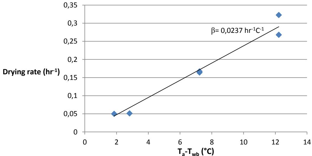
Figure 8: Drying rate as a function of the difference between the air temperature ( $T_a=20^\circ\text{C}$ ) and the wet bulb temperature ( $T_{wb}$ ).
