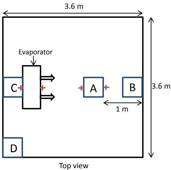
Positions of the temperature and relative humidity sensors
