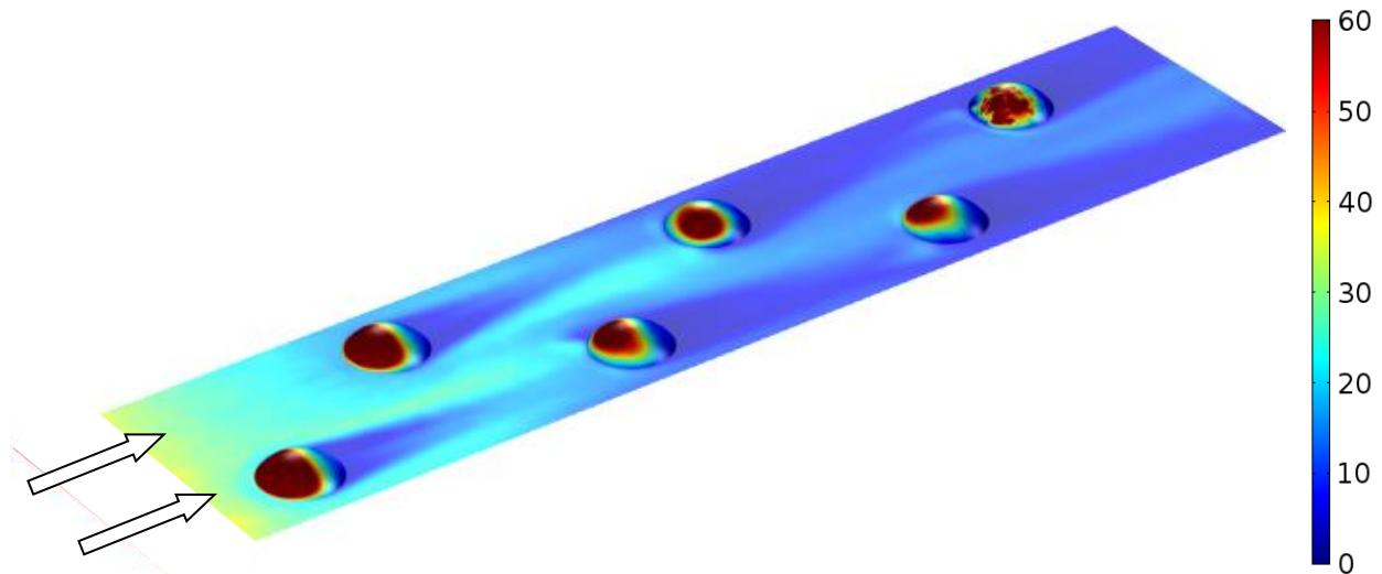
Fig. 3. Heat transfer coefficient ( $\text{W} \cdot \text{m}^{-2} \cdot \text{K}^{-1}$ ) on the air/water and air/plate interfaces
