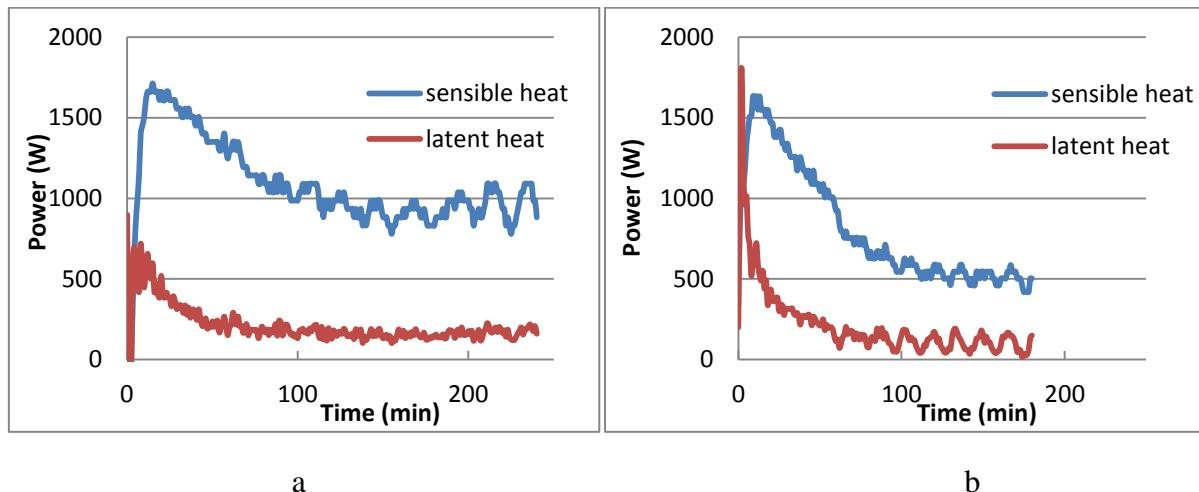
Figure 9: Evolution of the latent and sensible heat power during drying of 1 kg of water,
