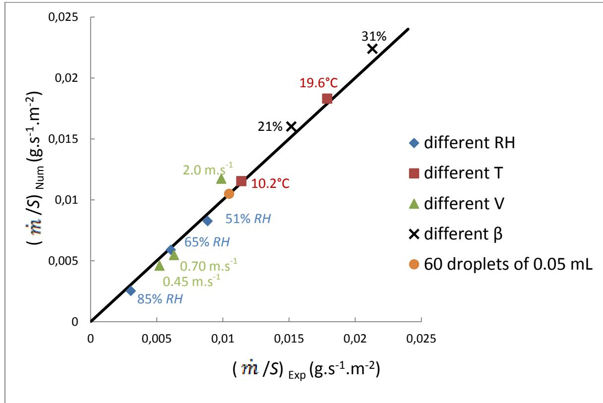
Low discrepancy between numerical and experimental values can be observed: high coefficient of determination  $R^2$  (0.98) and low average relative error (7.8%). This leads to conclude that in spite of the simplification of the numerical model (quasi steady-state, no radiation), it gives a good estimation of the evaporation rate during the period of constant wet surface.
