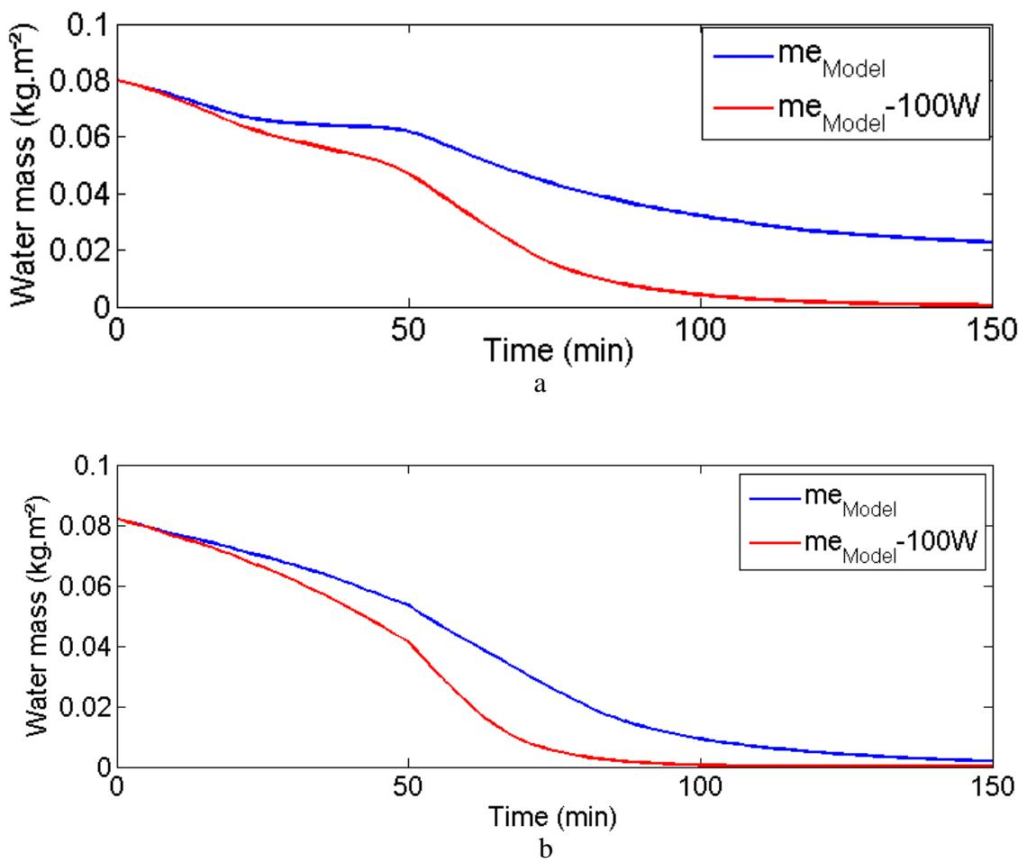
Figure 14: Comparison of the water mass evolution on the equipment with a 100W heat supply (red curve) and without a heat supply (blue curve). a- without a dehumidifier b- with a dehumidifier
