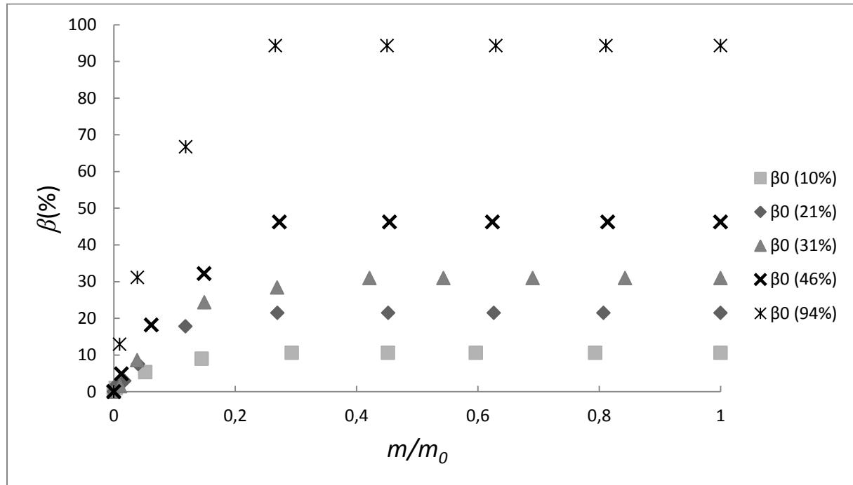
Figure 4: Evolution of the wet surface over the total surface ( $\beta$ ) in function of the water weight. Experiments performed inside a wind tunnel at a relative humidity of 51%, air temperature of 4.2°C and airflow velocity of 1.0 m.s<sup>-1</sup> with different initial values of  $\beta_0$ : 10, 21, 31, 46 and 94%
