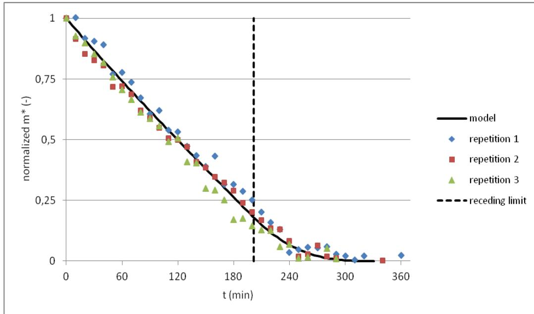
Fig. 4. Droplet mass evolution on stainless steel plate ( $m^* = m(t)/m_0$ ).
