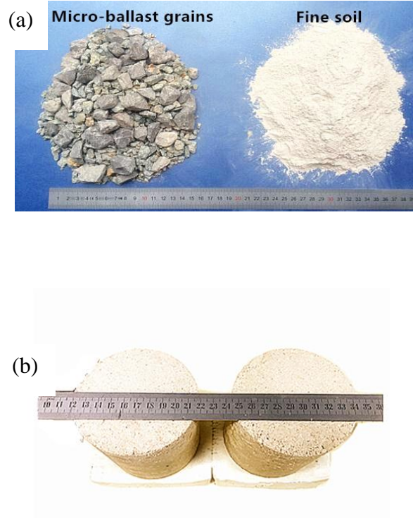
Fig. 5. (a) Preparation of fine soil and micro-ballast and (b) compaction of two soil disks
