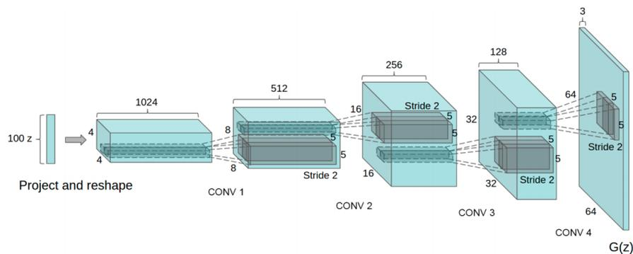
Figure 2.3: Fully convolutional generator architecture from (Radford et al., 2016) for adversarial image generation.
