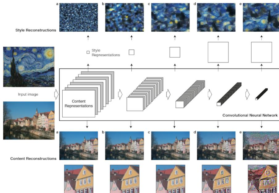
Figure 2.5: Using intermediate representations from a pretrained VGG network (Simonyan and Zisserman, 2014) to extract content and style information at different layers. These content and style features are used in style transfer and to define the perceptual loss (Johnson et al., 2016).
