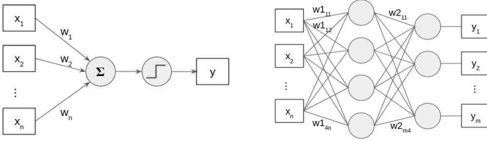
Figure 2.1: Visualization of the basic neural network architectures: the perceptron (left) and the multi-layer perceptron (right).
