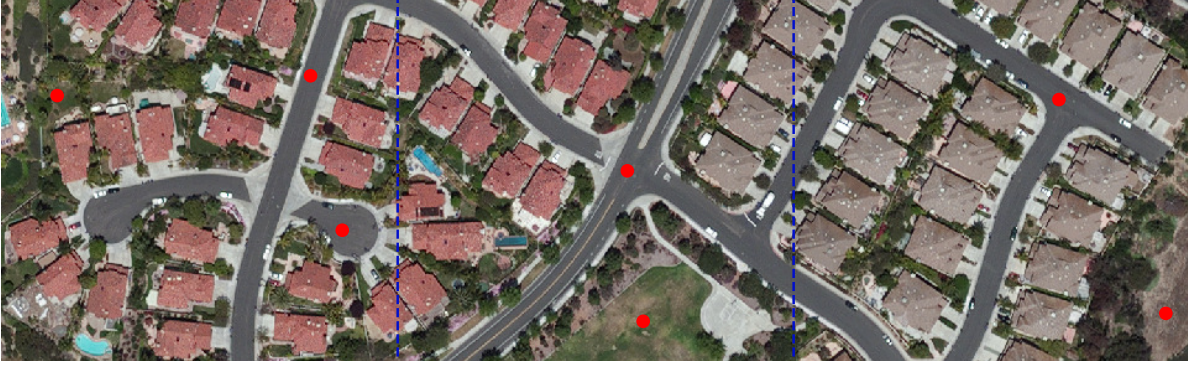
Figure 4.8 Image used to validate streaming version of the segmentation methods. The image has been split in three blocks (see blue dashed lines) and the blocks stream from left to right. As explained in Section 4.2 two consecutive blocks share a column of pixels. In red, the pixels used as markers for watershed-cut.
