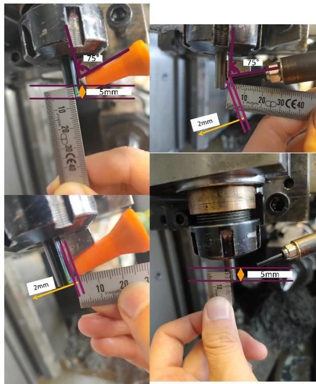
*Figure 37. Nozzle position in MWF and cryogenic assisted tribological tests*
