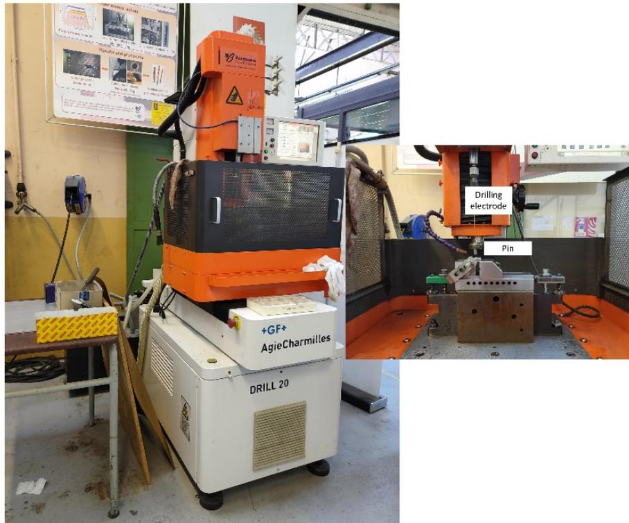
Figure 39. Drilling EDM machine and drilling position on pins and cutting tools
