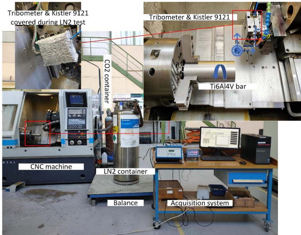
*Figure 36. The assembly of tribological tests*
