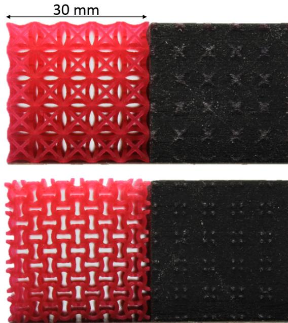
FIGURE 4.2 – Lattice samples of Hexaround and Warmuth structures after manufacturing (left side) shown in red and their composite counterparts filled with TangoBlack+ hyperelastic materials (right side)
