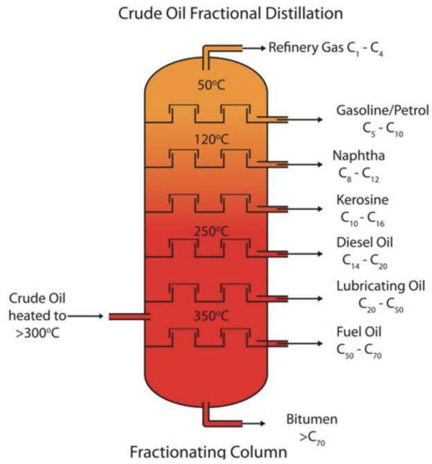
Figure 3.4: Simplified view of a distillation column
