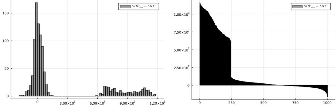
Figure 7.10: Left: Histogram of the score difference between  $\text{SDP}_{esp}$  and **Expert** over the assessment set. Right: Difference between  $\text{SDP}_{esp}$  and **MPC**, for the 1000 assessment scenarios, sorted
