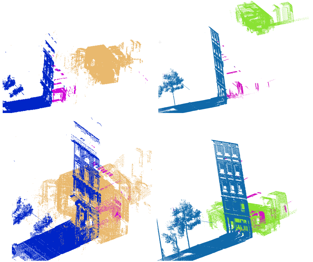
Figure 4.9: Result of the test of our algorithm on two pairs of indoor/outdoor scans, Top: the initial position of each pair, Bottom: The position of each pair after registration, pink points represent the indoor points detected from the outdoor scans.
