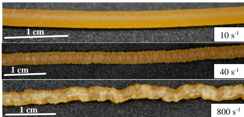
Figure 3.41 – Flow extrudates of SBR B at 100°C for a capillary die of  $L/D = 8$  and  $D = 2$  mm.
