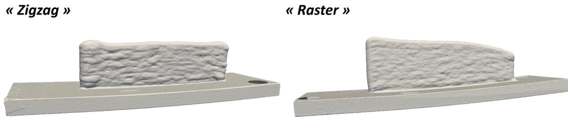
Figure 5.14 – 3D scan of the "Zigzag" and "Raster" 50 beads walls
