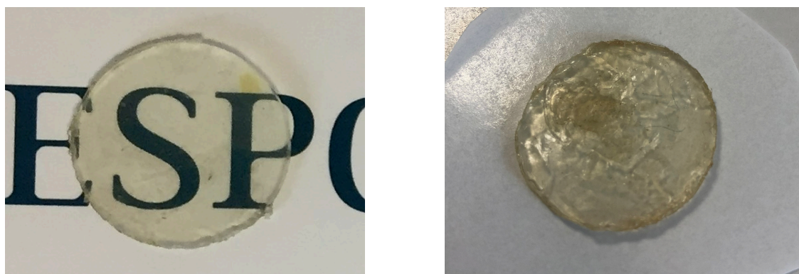
Figure 4.2: Pictures of Network 3a . Left: a sample directly after the processing. Right: a sample after two weeks at ambient conditions.
