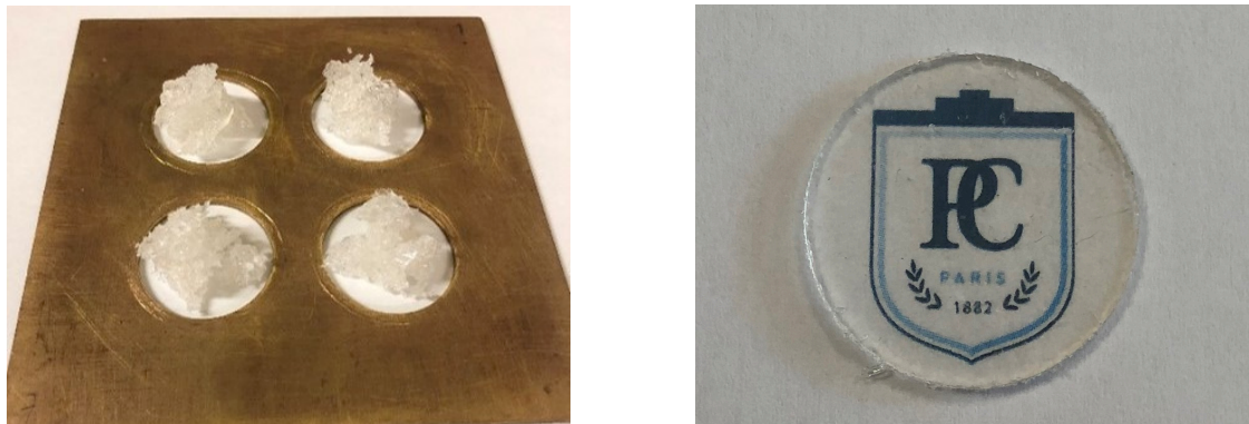
Figure 2.8: Pictures of Network 1 . Left: after crosslinking, before compression molding. Right: after compression molding.
