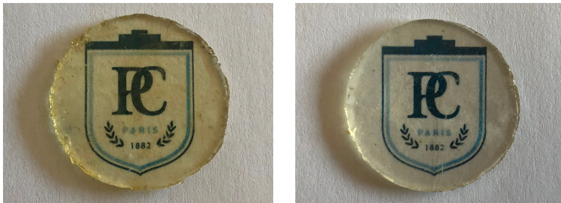
Figure 4.24: Pictures of Network 3c with \rho(\text{CL}) = 0.5\% after compression molding. Left: Sample Network 3c+RAFT . Right: Sample Network 3c-RAFT .
