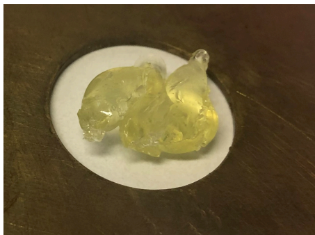
Figure 4.18: Picture of Network 3b after curing, before the compression molding.
