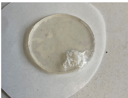
Figure 2.17: Sample of Network 1 after failed manual installation into the rheometer.
