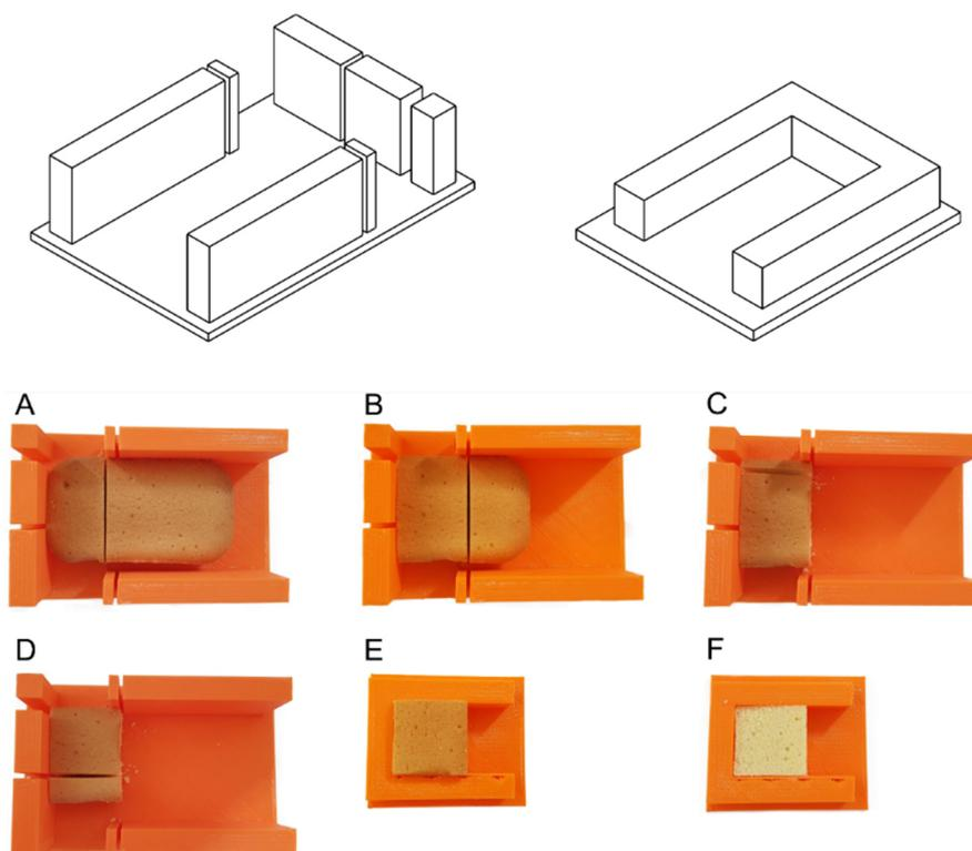
**Figure 41.** Cutting boards specifically designed to obtain a squared center piece of cake crumb with dimensions of 3 cm × 3 cm × 1 cm. The different steps of cutting are illustrated in the images A-F.
