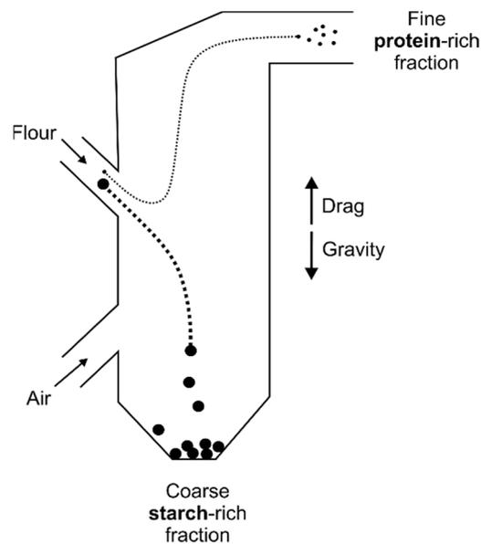
**Figure 14.** Principle of air classification (adapted from Shapiro *et al.* (2005)).
