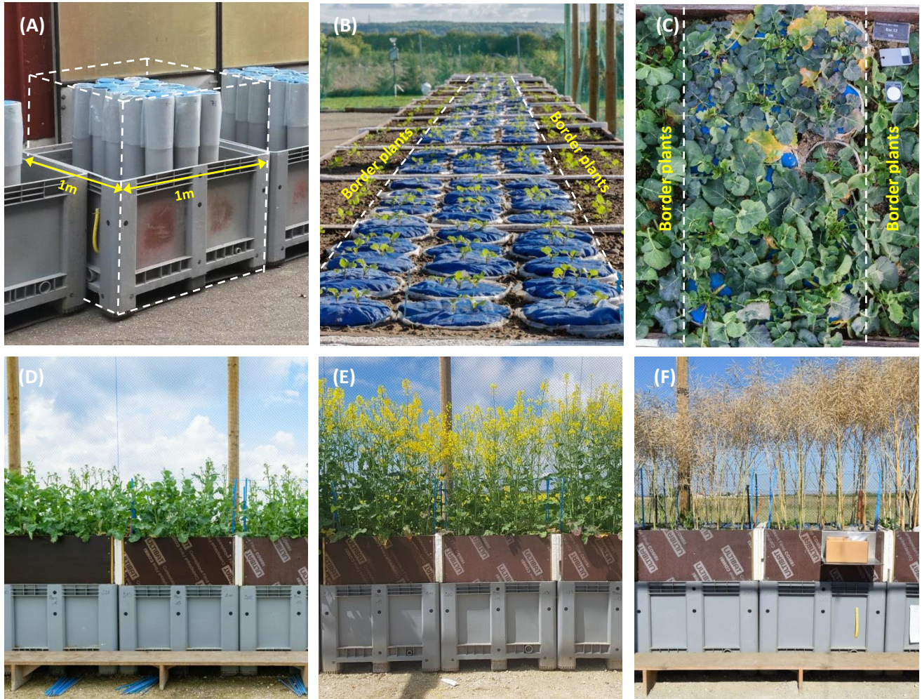
Figure I.3. Experimental device used for phenotyping N-use-efficiency-related traits during the whole crop cycle. Winter oilseed rape plants were grown under field-like conditions in a reconstructed canopy system (PERISCOPE device) allowing individual root and shoot measurements. Plants were grown in individual tubes 1 m high and 0.16 m in diameter, grouped into containers of 1 m 3 , placed outside and therefore submitted to field climate (A). Each tube was filled with substrate and regularly supplied with nutrient solution. In containers, the space between tubes was filled with soil to ensure the thermal insulation of root parts (B). Two rows of border plants were sown around the tubes to mimic bioclimatic field conditions. Six seeds were sown in each tube (B). After thinning, a single plant was kept per column, leading to a homogeneous canopy of 35 plants/m 2 (C, aerial view of one container), which were grown for the whole crop cycle until harvest (D, vegetative growth; E, flowering; F, seed filling and ripening). Photos correspond to the experiment conducted in Grignon in the 2017–2018 cropping season (GR18).
