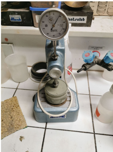
Figure 2.2 Views showing the determination of: (a) plasticity index (fall cone); (b) grain size distribution curve (sedimentometry).
