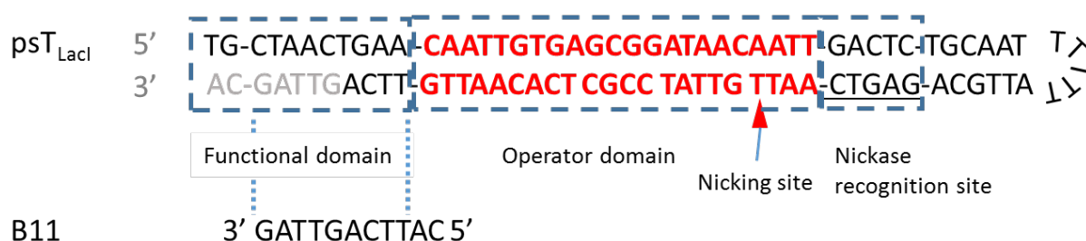
Figure 43 psT LacI detailed design. Here, going from right to left along the hairpin structure: polyT region and 6 bp, providing hairpin backbone; Nt.BstNBI recognition site (underlined); operator domain for TF binding (red), within which Nt.BstNBI nicking site is indicated (red triangle); functional region consisting of modified B11 signal sequence (shown standalone as well). The part of the sequence that was not chemically synthesised, but filled in by DNA polymerase upon reaction initiation, is shown in gray. Dashes are used for ease of interpretation.
