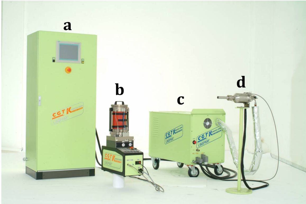
Figure 3.16: The cold spray system CGT Kinetics 3000. (a) control unit, (b) powder feeder, (c) gas heater, (d) gun.
