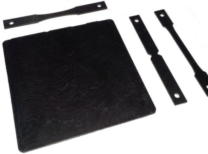
Figure 3.11: Photographic image of a VICTREX® PEEK™ 90HMF40 plate, as received.
