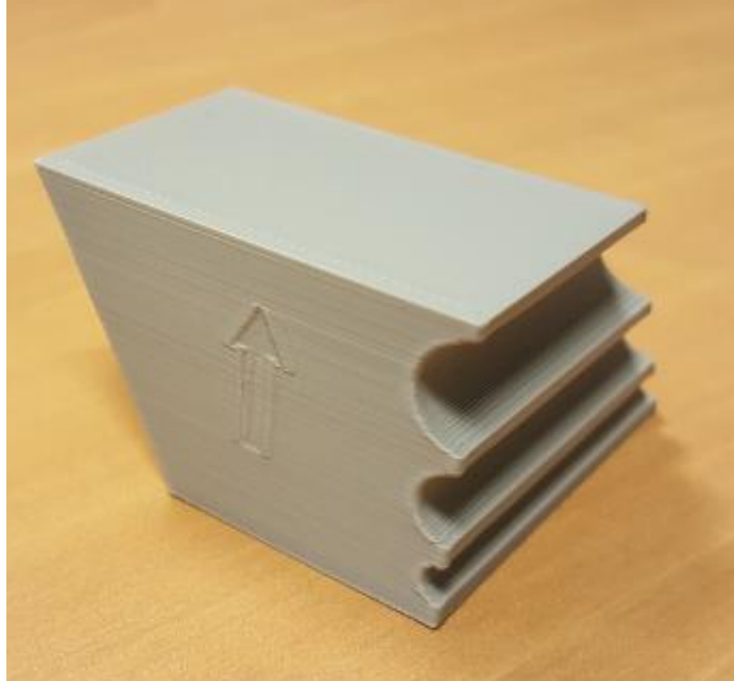
Figure 3.12: Photographic image showing one of the PA66 3D printed specimens.
