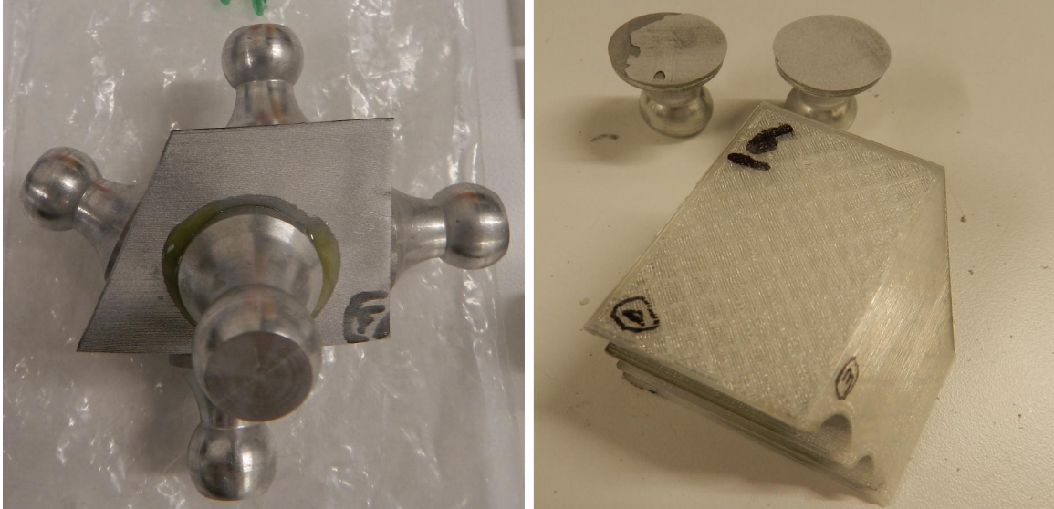
Figure 7.15: Photographic images of the pull-off test. On the left, sample preparation with all the pins glued to the metallized surfaces. On the right, the adhesive failure of an aluminum-PEEK coating.
